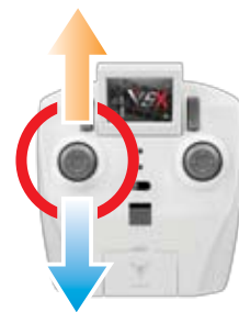
Push forward / backward to have the tank move in your desired direction
