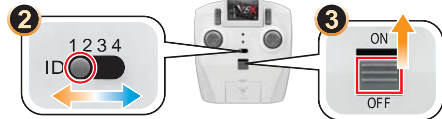
Set the ID of the controller to the tank's ID.
