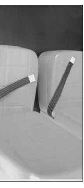
Wrap a piece of chrome MonoKote® trim sheet or foil around □ 3. Use the included elastic material to make the seatbelts. the ends to simulate buckles.
