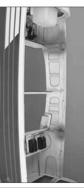
floor and sides. Also paint the formers in the fuselage that will not be totally concealed by the cockpit sides. floor where the seats will be glued down, then paint the cockpit □ 2. Use masking tape to cover the indentations in the cockpit
