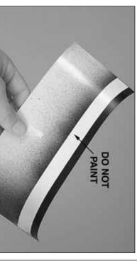
panel. Flat black is suggested. instrument panel. Paint the outside and inside of the valence get painted-this will allow for secure gluing to the valence panel 3/8" [9.5mm] from the aft edge so it will not 1. Use a strip of masking tape to cover the inside of the
