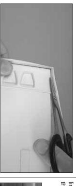
☐ 1. Use curved-tip plastic-cutting scissors to cut out the cockpit floor. After cutting, the floor should be a flat sheet with no lip around the edges. True the edges of the cockpit floor by sanding.
