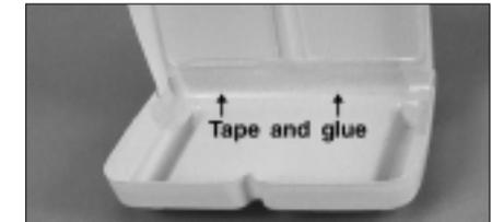
3. Insert the tabs of the rear seat back into the bottom half of the seat, then apply a piece of masking tape to the joint. The seat back should angle toward the rear of the cabin by a few degrees. Glue the seat back in position by "wicking" a few drops of thin CA into the joint from the back side. Remove the tape after the CA has cured.
