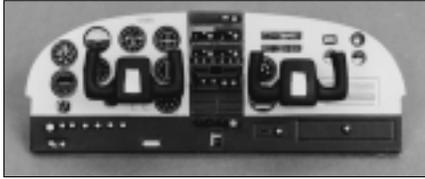
❑ 1. Carefully cut the **radios** and **fuel gauges** from the instrument decal included in your Top Flite Cessna kit and attach them to the **front** of the plastic instrument panel. Attach the remaining instrument decal pieces to scrap balsa or thin cardboard, then glue it to the **back** of the molded panel.
