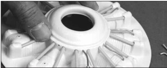
❑ 10. Insert the ignition leads into the cylinders. **NOTE:** Bend the ignition leads over the top of each cylinder so that they touch the backing. The ignition leads will be installed in the baffle later.
