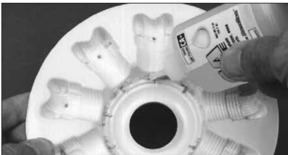
❑ 11. Turn the Radial over and apply a drop of CA to both ends of all pushrods and ignition leads.
