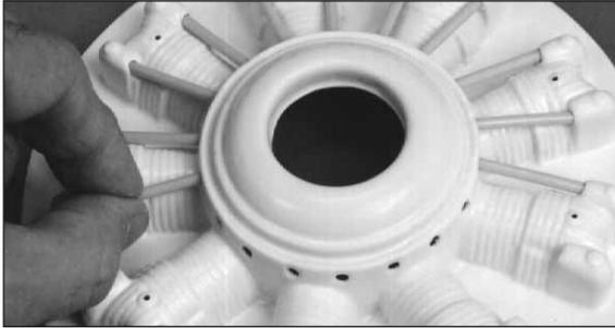
❑ 9. Insert the push pod tubes into the rocker arm covers and the crankcase as shown in the photo. They should protrude inside the Radial about 3/32" at each end of each piece. Don't worry about gluing them yet.
