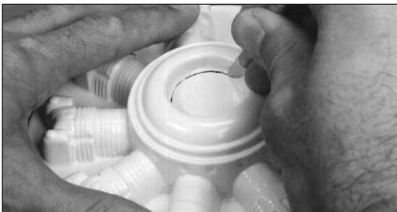
3. Cut away the prop shaft opening from the center of the Radial. Smooth the edges with a round file or drum sander.
