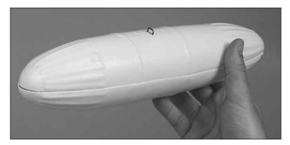
□ 11. Tape the two halves of the tank together in several places with masking tape. Glue the two halves together by wicking thin CA into the seam. Do not use accelerator as it will weaken the plastic.
