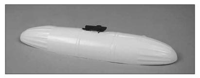
□ 6. Use 150-grit sandpaper to thoroughly roughen the inside of the tank where the release hook is secured. With the Release Loop inserted through the top half of the tank, test fit the Release Loop to the **Release Mechanism** to make sure there is no interference.
