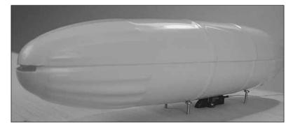
$\Box$  4. Install the tank on the Release Mechanism and tighten or loosen the #4 x 5/8" screws until you get the desired tank position. Ideally, the tank should have a slightly negative attitude so that it falls away from the airplane as soon as it is released. Wick thin CA on the screws to keep them from moving.
