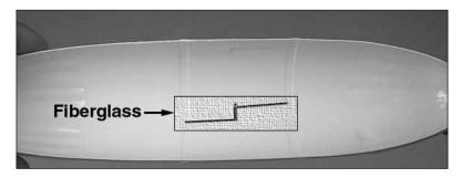
$\square$  8. Glue the Release Loop to the inside of the top half of the tank with 30-minute epoxy and the supplied 1" x 3" fiberglass tape. Allow the epoxy to cure.
