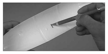
□ 5. Cut out the slot in the top half of the tank to allow the **Release Loop** to exit through the top of the tank from the inside.
