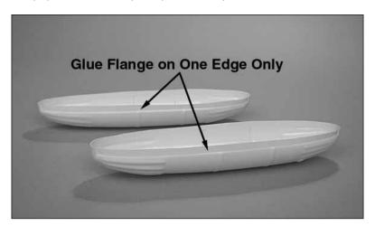
□ 2. Trim off the excess plastic to the cut lines on the inside of the tank with scissors or a hobby knife. Use 220-grit sandpaper to even up the edges of the glue flange.
