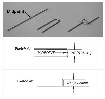
$\Box$  4. The supplied 0.046" dia x 3" steel wire needs to be bent by following these steps.
