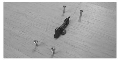
□ 3. Drill two 1/16" holes for the Release Mechanism's mounting screws. Using the sketch above as a sample, drill four holes for the drop tank positioning screws. The location of these screws will vary from airplane to airplane. Use thin CA to harden all the holes. Install the mechanism with two #2 x 3/8" screws included. Install the four #4 x 5/8" sheet metal screws included at the outer holes. These screws will be used to position the tank in the correct attitude.
