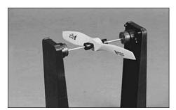
How to balance SMALL AND MEDIUM SIZE PROPELLERS: Slide the cones onto the balancer shaft with the tapered ends facing each other, trapping the propeller between the cones. The object
