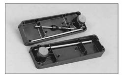
Place all components into the case halves in the positions shown in the photo. Press on the **ends** of the rods (not in the middle) when storing, to prevent bending. We recommend storing one base rod in each case half, for minimum case distortion.
