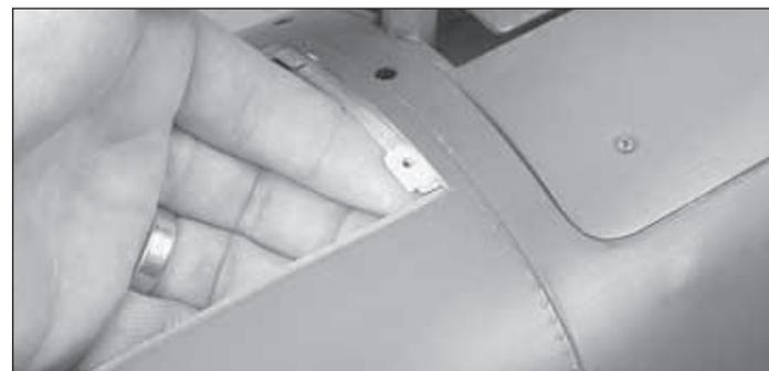
3. Install two (2) small pieces of 1/16" scrap ply under the inside edge of the nacelle to accept the hatch hold down screws. There are several aftermarket hatch latches that will work well also.
