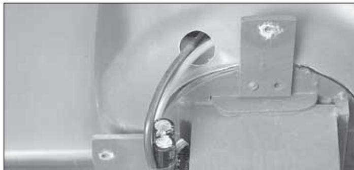
❑ 5. Drill a 1/2" hole in lower right front of the nacelle (from the pilots seat) to make an exit for the ESC leads.
