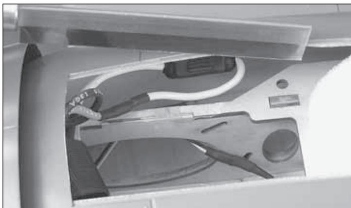
1. Cut the hatch in the bottom of both engine nacelles 4" x 3" between the back of the cowling and landing gear door with a thin razor saw. Keep this neat because you are creating a finished edge with the cut. Use masking tape along the edge while cutting to provide a guide and keep the edge clean.
