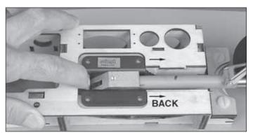
$\square$  4. Place the retract on the rails. With the strut retracted so it will be out of the way, position the retract **all the way back**, then drill four 7/64" [2.8mm] holes for the mounting screws. Mount the retract with four #6 x 1/2" [13mm] Phillips screws.
