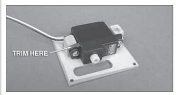
After mounting the rudder servos to the hatches, trim the front mounting tab of both servos as shown so the they fit in the hatch without contacting the top sheeting inside.
