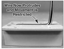
Use some material such as; (2) 3x30mm pieces of excess hook material included with the kit, a piece of plywood, a strip of rubber band, a strip of silicone sealant, to shim the channel of each block. Once the gear is secure, complete step #9.
