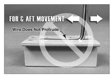
If there is movement fore or aft, or if the wires fail to protrude from the blocks, it is necessary to shim the channel of each block to restrict movement and ensure proper security.
