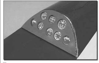
4. Glue the front instrument panel in place in the front of the cockpit.
