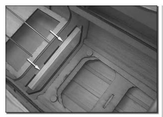
☐ 6. Locate the 6 x 6 x 90mm hardwood stick. Glue it in position on the fuselage former as shown. The stick should be glued on line with the visible tab slot.
