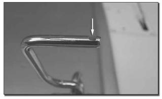
$\square$  10. File a flat spot onto the end of the axle.
