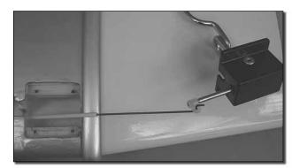
□ □ 8. Insert the wire from the retract into the tube. Using the tube as a guide, push the wire into the wing until the landing gear can rest on the landing gear rails. Remove the plastic tube.
