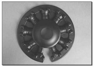
☐ 6. Cut away the portion of the dummy engine that will be in front of the engine cylinder. This is needed for proper cooling of the engine. When determining the exact location to cut, note that cylinders should be oriented as shown in the picture. We were able to cool the O.S. .91 by only cutting away a small portion of the cylinders as shown in the picture.
