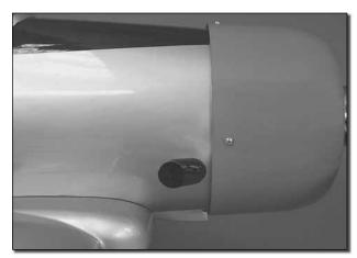
■ 8. Locate the black exhaust stack. Mark the location for it onto the fuselage. Cut a small amount of the covering away to create a solid place for gluing. Use 80-grit sandpaper and roughen the flat side of the stack that glues to the fuselage. Glue it to the fuselage.
