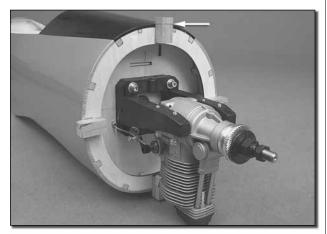
☐ 2. Epoxy each block to the front of the fuselage. Use the line you made as a guide for positioning the block. The line should be flush with the fuselage. One block should be mounted at each of the twelve, three, six and nine o'clock positions on the front of the fuselage.
