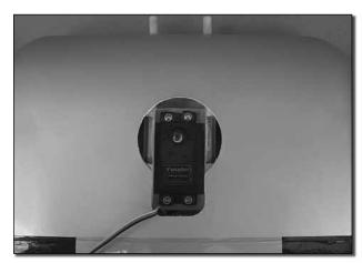
☐ 2. Install your retract servo between the mounting rail in the wing center section using the hardware that came with the servo.
