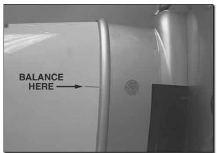
1. Use a felt-tip pen or 1/8" [3mm]-wide tape to accurately mark the C.G. on the top of the wing on both sides of the fuselage. The model should be
