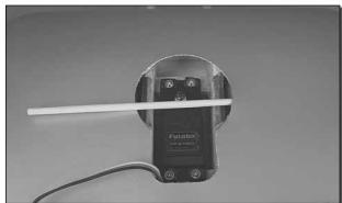
☐ 7. Insert the 12" [305mm] flexible plastic tube into the wheel opening, sliding it into the wing until it exits out at the retract servo.
