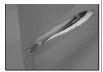
■ 8 Slide the end of the wire into the plastic tube at the stab opening in the fuselage.
