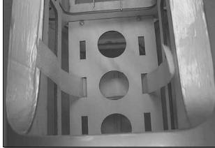
☐ 7. Cut two 6" [152mm] pieces of Velcro. Secure them to each other then insert the Velcro strap though
