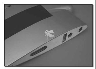
☐ 5. On each outer rib of the center section there is a string taped. Remove the tape and re-apply the tape and string onto the top of the center section.
