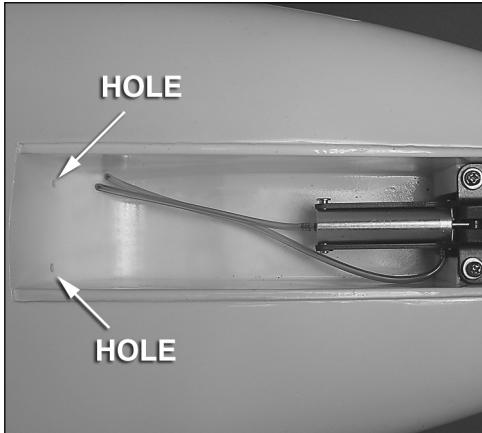
1. Located at the rear of the nose wheel compartment, are two small holes. Slide a tube into each hole.
