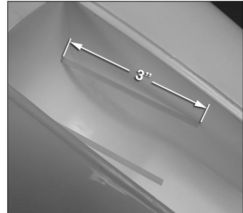
3. This should leave approximately 3" [76mm] of the tube extending into the nose wheel compartment. Secure the tubes to the hole in the nose wheel compartment with a couple of drops of thin CA. Do not glue the tubes to the elongated hole in the plywood bulkhead.
