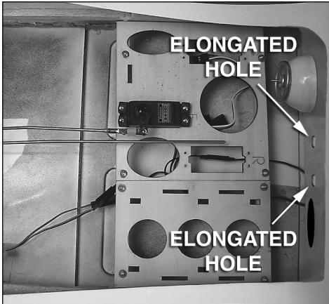
2. On the forward bulkhead you will see two elongated holes. Slide the tubes forward so they extend past the bulkhead approximately 1/4" [6mm].
