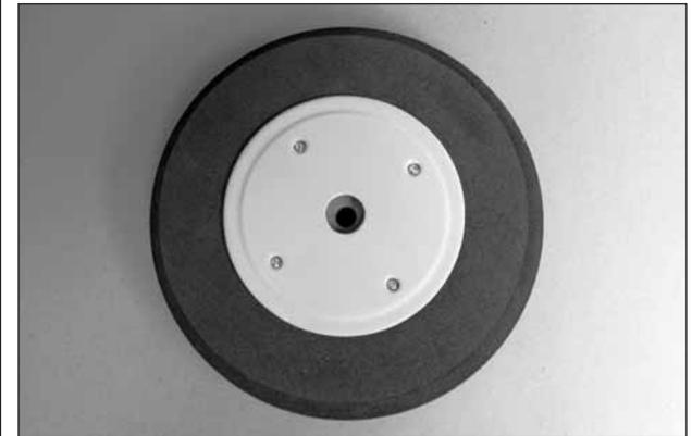
□ □ 15. Locate two of the wheel covers and the wheel. Screw the wheel cover with the large hole into the pre-drilled holes in the wheel with four 2mm x 4mm Philips head screws.
