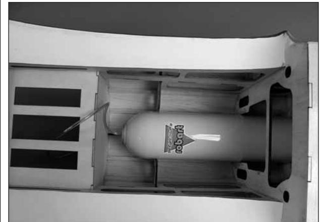
❑ 7. Install 18" [457mm] of air line onto the end of the air tank. Install the Robart air tank into the cradle in the fuselage. A couple of dabs of silicone sealant (such as Shoe Goo®) can be applied at the front to hold the tank in position, but still allow it to be removed if necessary. A plywood plate will be installed later to secure the tank.
