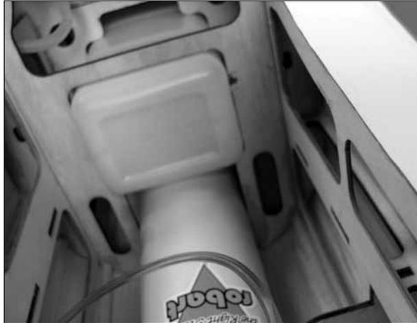
❑ 11. Install the fuel tank into the opening in the fuselage as shown. Feed the lines through the fuselage up to the firewall. Make sure when you insert the tank that the vent line is at the top of the tank.
