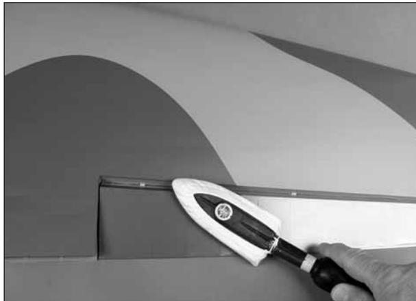
❑ 2. Use a covering iron with a covering sock on high heat to tighten the covering if necessary. Do this for all of the components of the model. Apply pressure over sheeted areas to **thoroughly** bond the covering to the wood.
