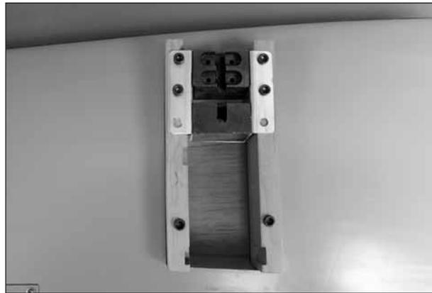
❑❑ 3. Install one of the **aluminum/fiber landing gear mounts** between the landing gear blocks. Temporarily secure the landing gear block and the landing gear mount with six 8-32 x 2-1/2" [64mm] socket head cap screws.
