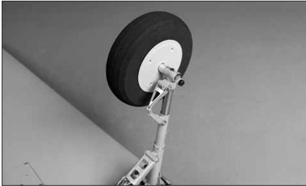
☐☐ 17. Insert the axle and wheel into the landing gear. Apply a drop of threadlocker onto the set screw; then, tighten the set screw against the flat spot on the axle.
