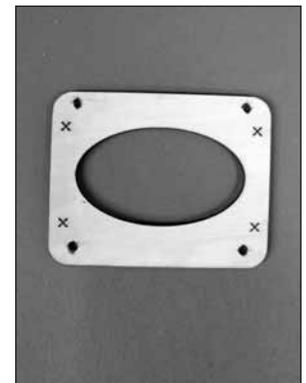
❑ 2. We have included 1/8" [3.2mm] plywood spacers to help space different engines out the required distance for the engine to fit the cowl. Drill a 3/16" [4.8mm] hole through the "+" marks on one of the plywood spacers. It's a good idea to fuel proof the spacer. This can be done by brushing a coat of 6-minute epoxy thinned with alcohol, or a coat of paint.
