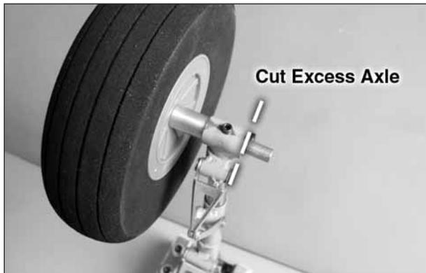
□ □ 12. Slide the wheel and axle into the landing gear. Make a mark on the axle where it needs to be cut to make it flush with the landing gear.
