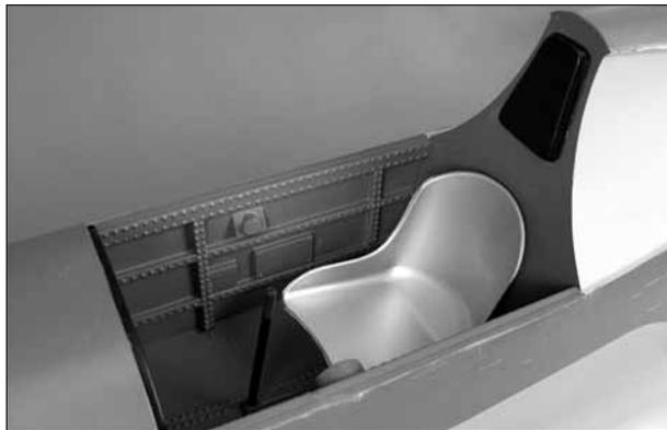
❑ 3. Glue the cockpit floor into the fuselage followed by the two side walls. When the glue has dried glue the seat to the pedestal molded into the cockpit floor.
