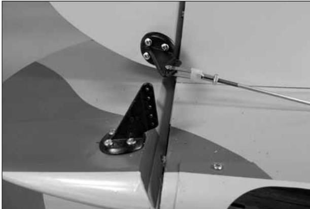
□ 4. Mount the control horns to the elevators and the rudder. Follow the same procedure used for the ailerons, by drilling  $3/32$ " [2.4mm] holes and using #4  $\times$   $1/2$ " [12.7mm] sheet metal screws. Attach the elevator clevis in the third hole from base of the control horn. Don't forget to harden the holes with thin CA after first installing, then removing the screws.
