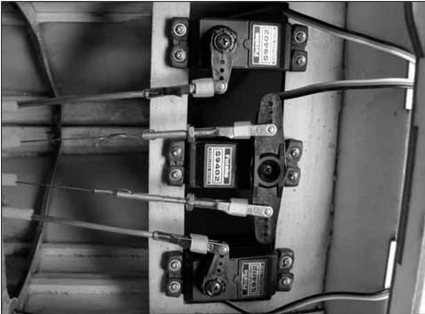
❑ 8. Center the servo arm and the tail wheel gear. Install a swage on each cable, securing it following the same procedure used on the tail gear. Use pliers to crimp the swage tightly on the cable.
