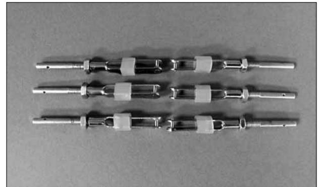
□ 7. Thread a 4-40 nut and a 4-40 metal clevis, 12 turns, onto each of six 4-40 rigging couplers. Install the clevises on the tailwheel steering servo arm in the holes  $5/8$ " [15mm] from the center of the servo arm.
