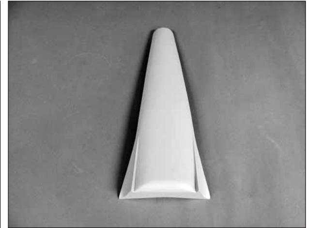
❑ 6. Mount the wing to the fuselage with the two 1/4-20 x 2" [51mm] nylon wing bolts. Locate the fiberglass belly pan. Place it on the wing. With a fine-tip felt pen, mark the location on the wing for the belly pan.
