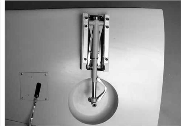
☐☐ 3. Install the right side **landing gear** between the mounting blocks. The landing gear fits between the blocks best if you install it with the gear retracted. Mount the landing gear and the blocks with six 8-32 × 2-1/2 [64mm] socket head cap screws, #8 flat washers and #8 lock washers.
