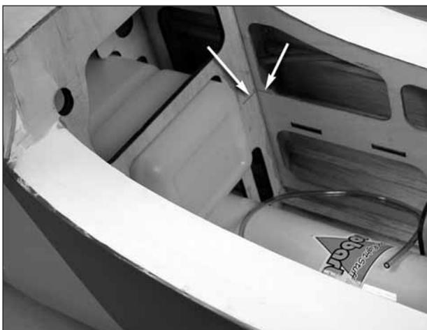
❑ 23. With the servo tray resting in place on the air tank, make a mark on the fuselage formers to show the location for the tray at each of the four corners of the tray.
