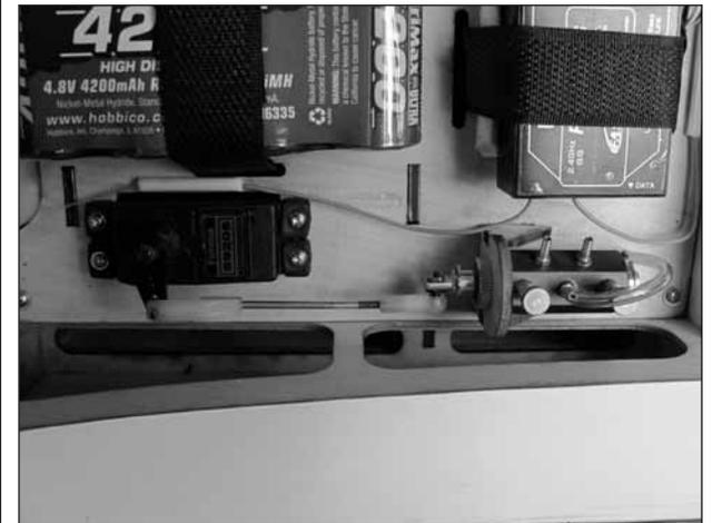
❑ 30. Thread a nylon ball link onto one of the .074 x 6" [152mm] wires threaded on one end. Snap the ball link onto the ball on the air control valve. Center the servo and the air control valve. Make a mark on the wire when it is aligned with the outer hole in the servo arm. Make a 90 degree bend on the mark. Cut off the excess wire 3/8" [9.5mm] above the bend. Insert the wire into the outer hole of the servo arm. Install a Faslink™ onto the wire to secure it to the servo.
