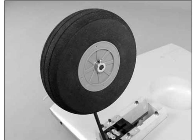
□ □ 8. Slide a 6mm [15/64"] wheel collar onto the axle followed by a 5/8" [16mm] long aluminum tube. Slide the wheel onto the axle. Insert a 3mm × 5mm phillips head screw into another 6mm wheel collar and then secure the wheel collar to the **end of the axle**.
