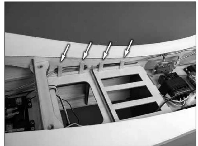
□ 34. Route the air lines from the tailwheel through the fuselage and secure them. We used some scraps of balsa to secure them to the fuselage as shown.
