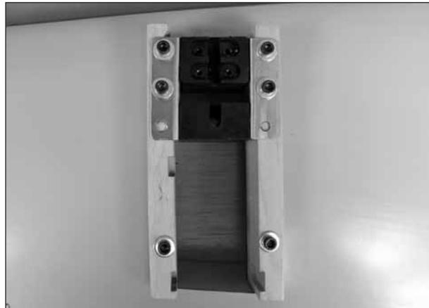
❑❑ 5. Double-check both of the landing gear block installations to be sure they are correct. When you are satisfied with the installation, remove the bolts from the right wing panel. Mix a 1/2 ounce [4 drams] of 30-minute epoxy. Use an epoxy brush to apply a film of glue to the bottom of the landing gear mounting blocks and to the rails in the wing as well as the sides of the box the mounts slide into. Be careful not to get glue into the blind nuts. If you get glue into the threads of the
