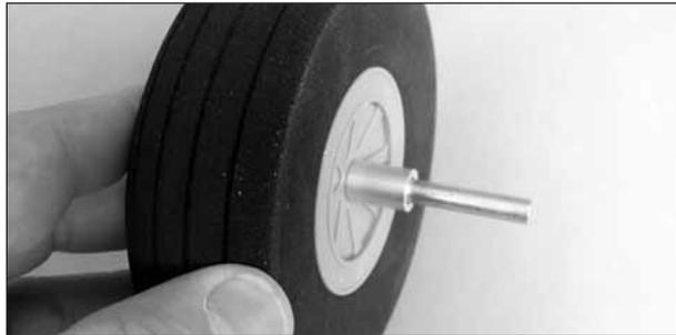
□ □ 11. Locate a wheel, the 5/8" [16mm] long aluminum tube and the axle included with the landing gear. Slide the axle into the wheel and slide the aluminum tube over the axle.
