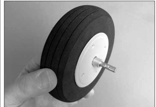
□ □ 16. Slide the axle into the wheel from the side without the wheel cover; then, slide the aluminum tube over the axle.
