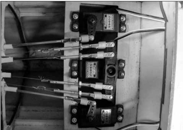
❑ 11. Attach each clevis to the outer hole of the servo arm.
