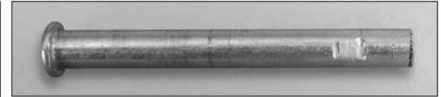
□ □ 14. Determine where the set screw makes contact with the axle. Make a flat spot on the axle with a file or motor tool.
