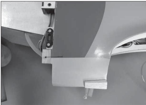
❑ 6. Place the block against the fuselage where shown. Mark the area and then cut the covering away from the fuselage using the same technique used for removing covering on the model in earlier steps. Glue the blocks in place on both sides of the fuselage. Fuel proof the blocks with paint or a light coat of thinned epoxy.
