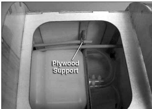
❑ 22. In the front of the fuselage, glue the plywood support for the choke tube to the former. Once the glue has cured cut off the portion of the plastic tube between the firewall and the plywood support as shown in the photo.
