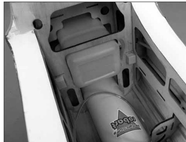
❑ 24. 1/8" [3.2mm] below the marks you made make another line. Glue a 3/8" x 1/2" x 5/8" [9.5mm x 13mm 16mm] hardwood block so that the top of the block is aligned with the new line you just made. The tray will rest on and be screwed into the blocks. Once the glue has cured place the tray onto the blocks. Drill a 1/16" [1.6mm] hole through the holes in the corners of the tray into the blocks and then remove the tray.
