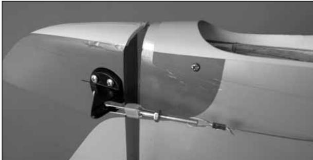
❑ 12. Attach the remaining two clevis assemblies into the middle hole of the rudder control horn on each side of the rudder. Center the rudder and the rudder servo. Attach the wire to each of the clevis assemblies using the same technique used on the other clevis assemblies.
