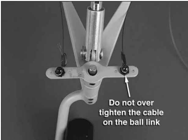
❑ 8. Now pull on the long end of the cable to reduce the size of the first loop. Slip the loop over one of the ball link balls on the steering arm. Tighten the loop until it is small enough to remain secure on the ball, yet may still be pried off. Squeeze the swage with pliers. Connect the other cable to the other ball link ball the same way.
