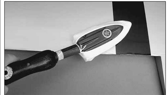
3. If necessary, use a covering iron with a covering sock to go over the wing, flap and aileron to remove any wrinkles. The best method to remove the wrinkles is to glide the iron over the covering until
