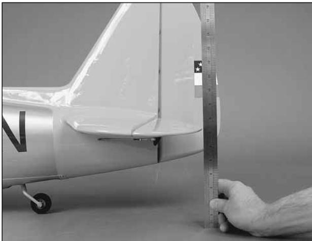
❑ 1. Use a box or something similar to prop up the bottom of the fuselage so the horizontal stabilizer and wing will be level. Hold a ruler vertically on your workbench against the widest part (front to back) of the trailing edge of the elevator. Note the measurement on the ruler.
