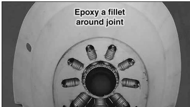
❑ 9. Before gluing, use sandpaper to roughen the gluing area inside the cowl. Clean the area with a paper towel dampened with denatured alcohol. Mix approximately 1/2 oz [14.7cc] of 30-minute epoxy. For a stronger joint, add some milled fiberglass to the epoxy. Apply epoxy to the edge of the engine assembly and insert it in the cowl. Use the remaining epoxy to create a fillet around the edge of the assembly.
