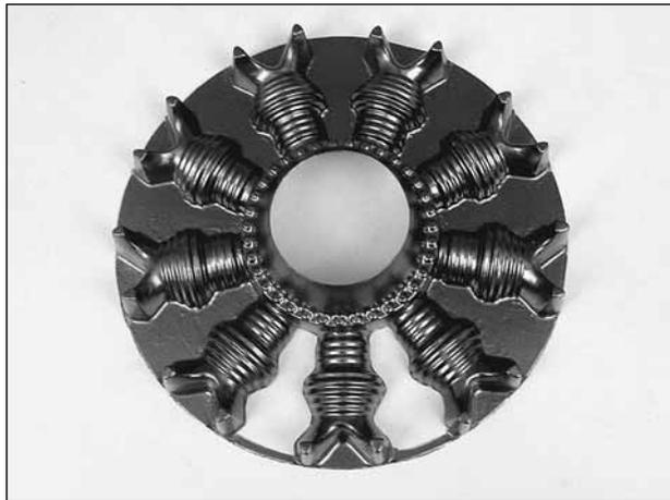
❑ 4. Cut out two openings between the cylinders and the center of the plastic radial engine. The center hole needs to be large enough to clear the drive washer of the gas engine.
