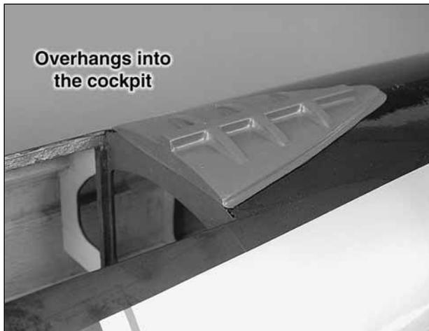
❑ 6. Trim and glue the canopy track to the top of the fuselage. Note that the front of the canopy track overhangs into the cockpit.
