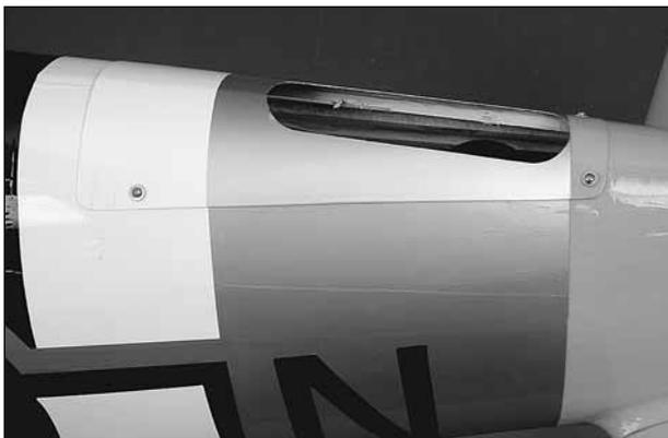
❑ 9. The tail gear retract cover can be permanently installed using CA glue or with screws. If CA glue is used it will be difficult to remove the cover and access the retracts if needed. To install the cover with screws, tape a piece of paper to the fuselage at each corner of the tail gear opening. Place a mark on the paper
