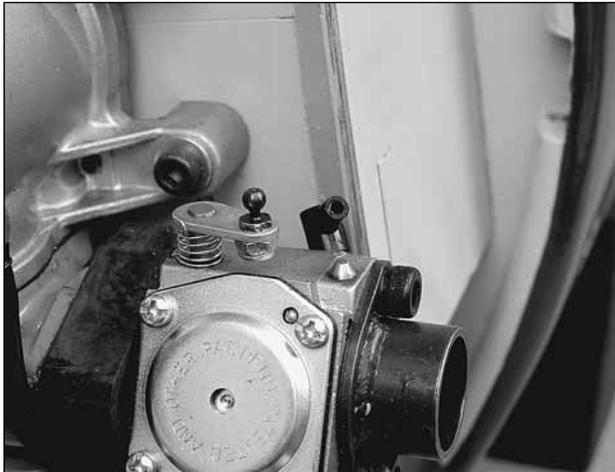
❑ 3. Install a 2-56 ball link ball on the throttle arm of the carburetor. Secure the ball link ball with a 2-56 lock nut.
