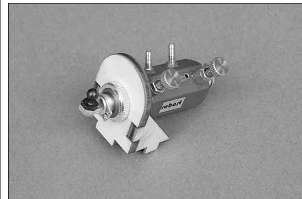
❑ 4. Assemble the retract control valve mount and install the retract control valve. Install a .080 ball link ball and .080 nut on the valve. Be sure to use a drop of threadlocker on the threads of the ball link ball.
