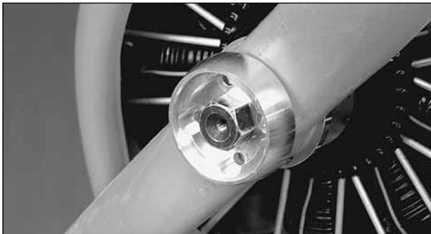
❑ 2. The included aluminum prop hub was designed to be used with the DA-50 or the Fuji-Imvac BT-43E1-2 gas engines. Bolt the include prop hub in front of the propeller in place of the prop washer.
