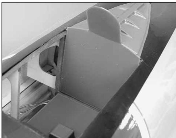
❑ 7. Glue the armor plate to the back of the cockpit.
