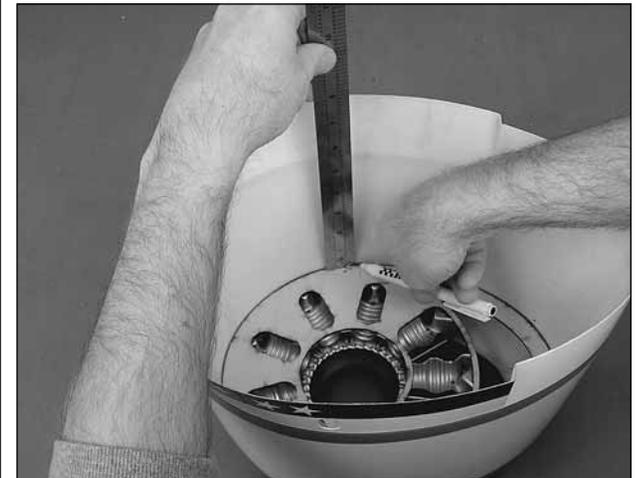
❑ 8. Test fit the radial engine assembly in the cowl. Position it so it is centered and equal distance from the edge of the cowl. Mark the location on the inside of the cowl. This will help you reposition the engine once you have applied epoxy to the engine assembly. Use masking tape to hold the dummy engine in position and test fit the cowl on the fuselage over the gas engine.
