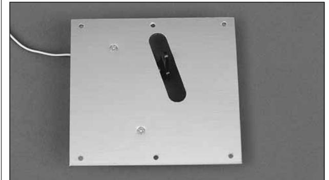
6. Drill 1/16" [1.6mm] holes through the blocks at the two hole locations on the top of the aileron servo hatch. Install two #2 x 3/8" [9.5mm] flat head sheet metal screws to secure the servo mounting blocks to the aileron servo hatch. Use thin CA to harden the screw threads.
