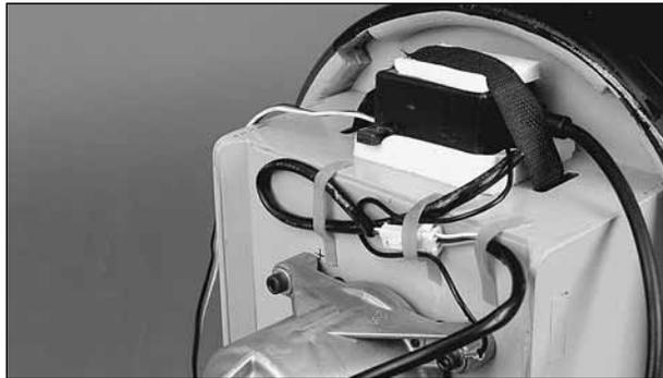
❑ 10. Place the ignition module on a piece of R/C foam rubber and secure it to the top of the firewall box with hook and loop material. Rubber straps, cut from a rubberband (not included) can be glued to the firewall box to hold the excess wires.
