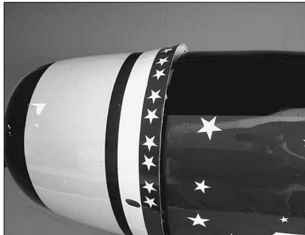
❑ 11. Test fit the cowl over the engine. Install the recommended propeller on the engine. Adjust the position of the cowl so that the dummy radial engine is centered on the drive washer and the propeller clears the front of the cowl by 1/8" [3.2mm]. The cowl mounting brackets should be approximately 1/8" [3.2mm] inside the edge of the cowl.
