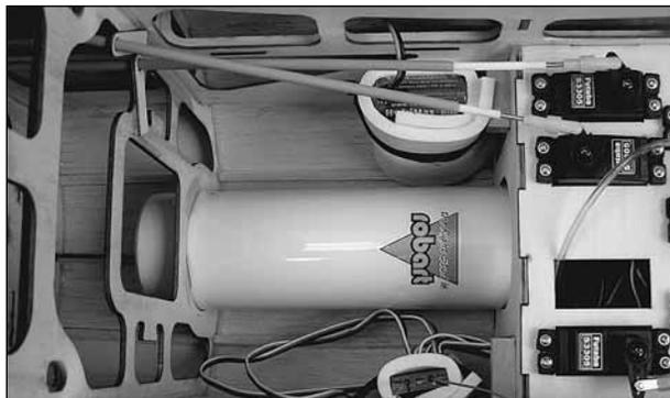
❑ 1. Attach a 12" [305mm] piece of airline tubing to the pressure tank. Insert the pressure tank into the fuselage. A couple of dabs of silicone sealant such
