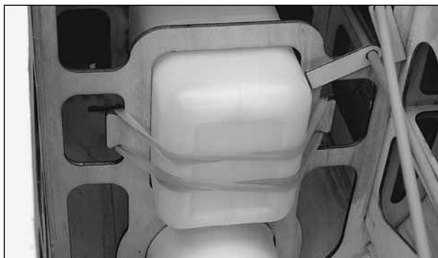
❑ 5. Determine how you want to run the fuel line and drill holes where necessary in the firewall. Install fuel line on the three tubes from the fuel tank. Insert the fuel tank in the fuselage making sure the vent tube is towards the top of the fuselage. Connect the fuel
