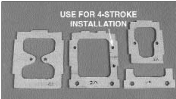
□ 3. Drill a 3/16" [4.8mm] hole in the punch marks on formers **F-2A, F-2B, F-4A** and **F-5A**. These will accommodate the pushrod installation as we build the fuse.
