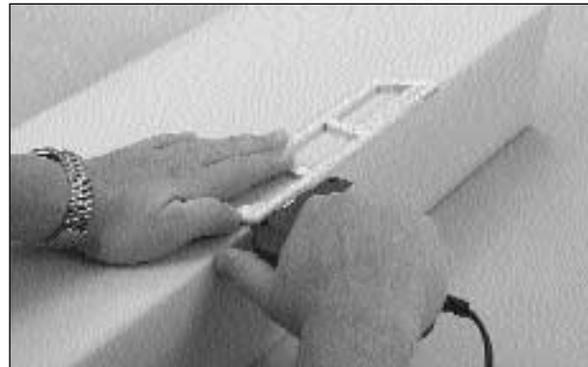
*To cut the hinge slot place the blades onto the wood where you want the slot. Lightly press the teeth into the wood. When you are satisfied with the location press the button on the handle and the blades will cut easily into the balsa wood.*
