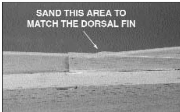
□ 36. After the supports are glued in place, slide the fin assembly between the fin supports. Sand the fin
