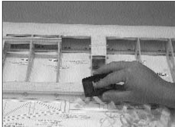
□ 35. Use a razor plane to shape the 9/16" x 7/8" [14.3 x 22.2mm] TE that you glued in place in step 9. Shape the TE to match the airfoil of the ribs.
