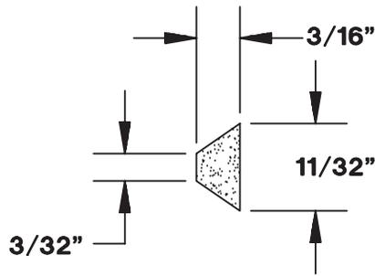
❑ ❑ 4. Cut a shaped 18" [457mm] balsa **flap spar** to fit between flap ribs W2A and W8A. Test fit, then glue the flap spar in the notches of the flap ribs.
