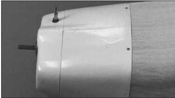
❑ 13. Remove the cowl and cut the hole for the needle valve. Start with a small hole. Mount the cowl to the fuselage and check your accuracy. Enlarge the hole while you simultaneously change its position if necessary.
