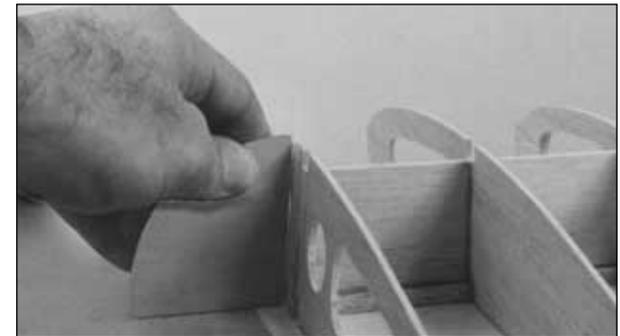
□ □ 9. Place rib W2 back onto the assembly. Align W2 with the dashed line depicting where it contacts the plan. Use the die-cut 1/8" [32.mm] plywood **dihedral gauge** to set W2 at the correct angle. Glue it to the bottom spar and the spar web. Glue W2 to the aft inner spar using the dihedral gauge to set it at the correct angle.
