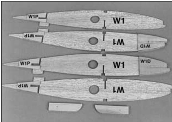
□ 2. Prepare two **W1** ribs as follows: Use thick or medium CA to glue two die-cut 1/8" [3.2mm] plywood **dowel rib doublers W1D** and one **bolt plate rib doubler W1P** to the sides of each die-cut 1/8" [3.2mm] balsa **ribs W1** as shown on the plan. Pay careful attention to which sides of the ribs the doublers are glued.
