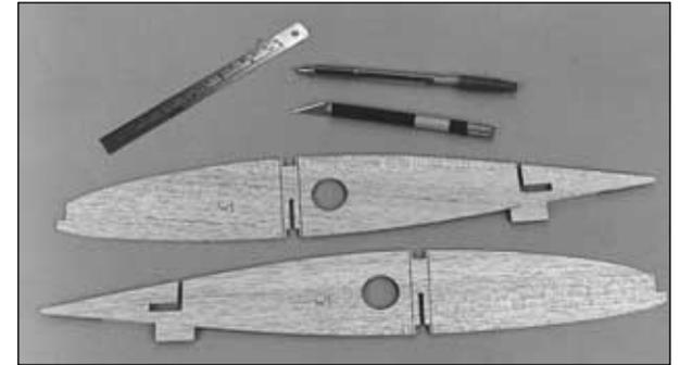
□ 8. With a straightedge and a ballpoint pen mark two vertical lines 1/16" [1.6mm] ahead of and behind the spar notches on the **outside** of both of the W1 ribs, that have only the W1P doublers glued to them. Use a sharp hobby knife to cut halfway through the balsa along the lines. This section of balsa will be removed to accommodate the spar joiners when it is time to join the wing.
