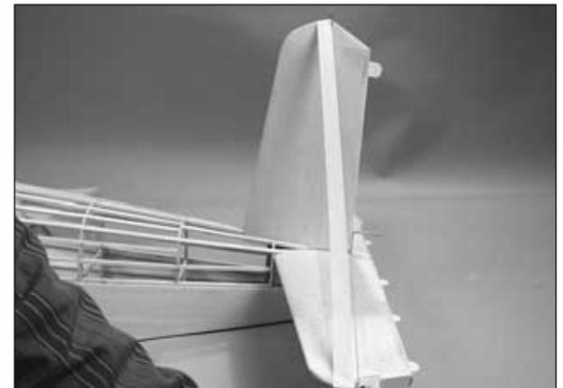
❑ 4. Mix some 30-minute epoxy. Glue the basswood stick into the fin making sure to put epoxy on the end of the stick that touches R2 inside the fin. Glue the fin and stick to the top of the stab and to former F10.
