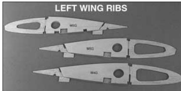
□ F8. Prepare a set of **left** wing ribs the same way but **use the photo above** to make sure you glue the doublers to the correct side of the ribs.
