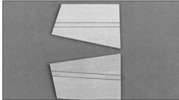
❑ F2. Place the braces over the **nose gear detail** on the plan. Mark the location of the 1/4" [6.4mm] plywood landing gear rails onto the braces.
