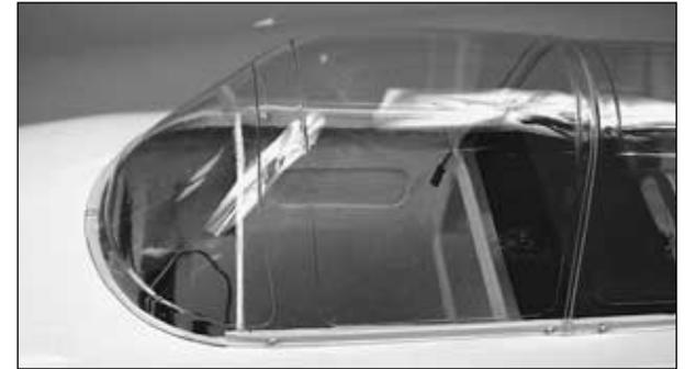
❑ 4. Cut the front canopy out on the cut lines and fit the canopy into place on the fuselage. We held the front canopy in place with five #2 x 3/8" [9.5mm] sheet metal screws.
