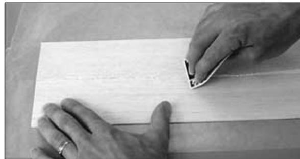
**D.** Use a credit card or a piece of thin plywood to simultaneously **press** the sheets flat as you squeegee the excess glue from the seam. Wipe the glue off your squeegee with a paper towel or a stick of wood. Immediately proceed to the next step.
