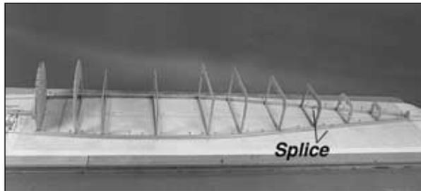
❑ 4. Position but do not glue formers **F1** through **F11** on the side stringers so the embossed names on the formers face forward. Adjust the stringers as needed. *Are your 3/16" [4.8mm] pushrod holes drilled?*
