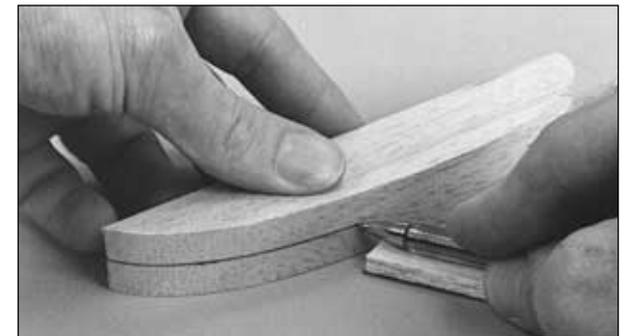
❑ 40. Draw a centerline all the way around a 3/4" [19mm] shaped balsa **stab tip block**.
