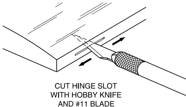
❑ 36. Cut the hinge slots on the centerlines of the elevators and the stab where shown on the plan.
