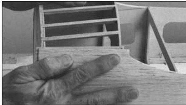
❑ ❸ 3. Reposition the side sheet on the fuse. Mark and trim the front bottom of the side sheet 1/8" [3.2mm] above the bottom of the balsa front fuse doubler.
