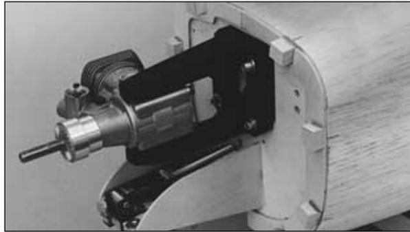
❑ 6. Test fit eight 1/2" x 1/2" x 5/8" [12.7 x 12.7 x 15.9mm] maple **cowl mount blocks** in the notches in the cowl ring. Sand the blocks so they match the shape of the cowl. Glue them in place. Mark the center of each cowl mount block on the fuselage. Test fit the cowl to the fuselage to make sure none of the blocks interferes with the cowl.
