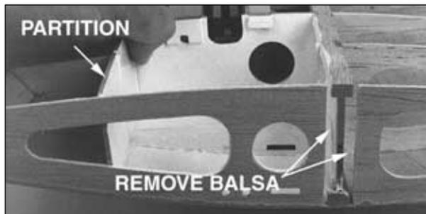
❑ 2. Remember where you cut **partway** through ribs W2 on both wing panels 1/16" [1.6mm] ahead of and behind the spar notches? Use a hobby knife or a fine razor saw to cut the rest of the way through rib W2 on the right wing panel and remove the balsa within the area you cut.
