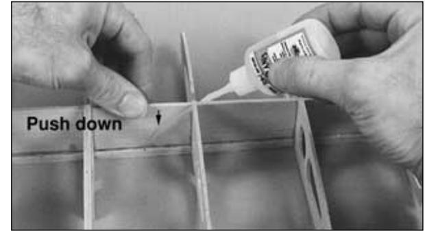
□ □ 8. Use medium or thin CA to glue all the joints. Use the CA sparingly at this stage of construction and do not build up fillets. This will allow you to realign parts if necessary and keep you from gluing the jig tabs to the ribs. We will remind you to reinforce all glue joints later.
