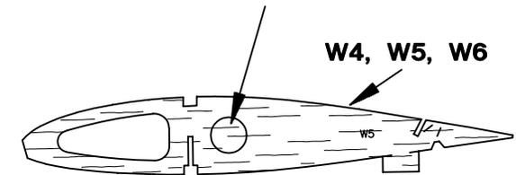
**Note:** If you are going to install retracts, don't punch out the round *lightening hole* in the die-cut 3/32" [2.4mm] balsa **wing ribs W4, W5 and W6**. Instead, apply thin CA around the lightening hole to glue it in place.
