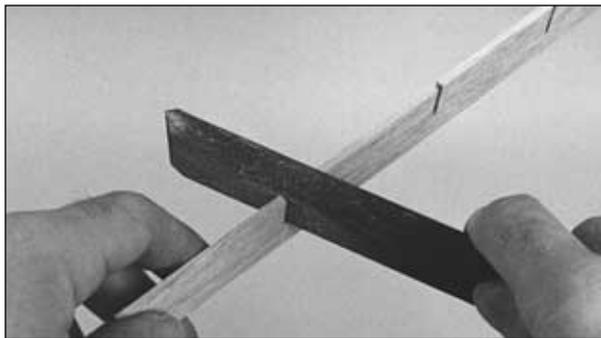
□ □ 4. Test fit the die-cut 1/8" [3.2mm] balsa **aft inner spar (W18)** into the notches of ribs W2
