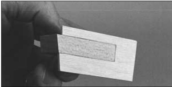
❑ 1. Bevel the end of both 1/2" x 1" x 2-1/4" [12.7 x 25.4 x 57.2mm] maple **wing bolt blocks** so they match the angle of the die-cut 1/8" [3.2mm] plywood **wing bolt block holder**.
