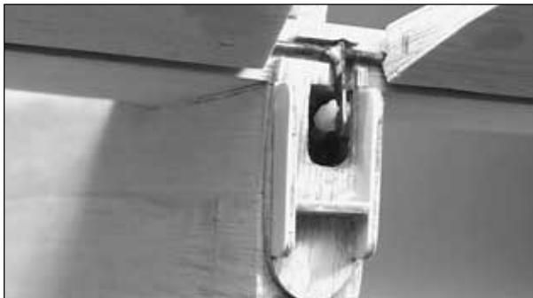
❑ 2. Glue the die-cut 1/8" [3.2mm] plywood **tail cone mounts** to the tail cone former.
