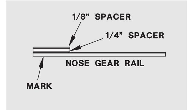
❑ R2. Glue one 1/4" x 9/16" x 2-1/4" [6.4 x 14.3 x 57.2mm] plywood **rail spacer** and one 1/8" x 9/16" x 2-1/4" [3.2 x 14.3 x 57.2mm] plywood **rail spacer** on the end of both rails that you made the mark on, but on the other side of the rail.
