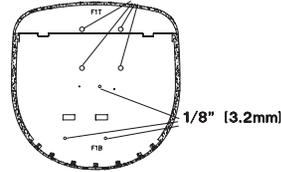
❑ 6. Drill the correct size holes through the punch marks on the front of the firewall as shown in the sketches above. Tightly hold a **thick** block of wood on the back so the drill does not split the wood when it comes through.
