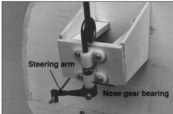
□ F8. Mount the nylon **nose gear bearing** to the nose plate with four 4-40 x 1/2" [12.7mm] screws. Enlarge the holes in the nose gear bearing for the nose gear strut with a #10 drill bit (if you don't have a numbered drill set, an 13/64" [5.16mm] drill bit will work too).
