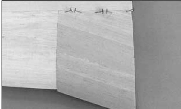
❑❑ 8. If you haven't already done so, glue two more 3/32" x 3" x 30" [2.4 x 76 x 762mm] balsa sheets together for the **forward inner skin**. From that sheet, cut a piece that fits between ribs W2 and W4 and glue on a third piece cut from leftover 3/32" [2.4mm] balsa to fill up the rest of the space. Note that the grain direction is parallel to the leading edge between ribs W2 and W4. Trim the sheet to fit the wing. Glue it in position.
