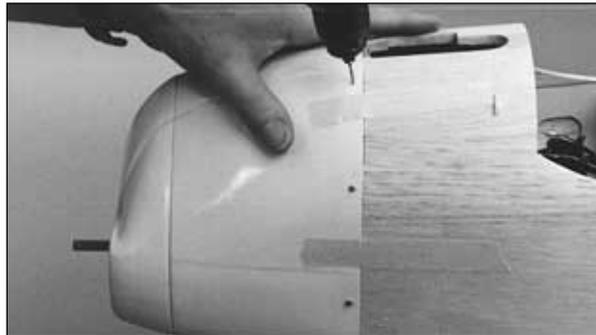
❑ 7. Securely tape the cowl to the fuselage. Using the marks as a guide, drill 1/16" [1.6mm] holes through the cowl and the cowl mount blocks 1/4" [6.4mm] in front of the aft edge of the cowl.
