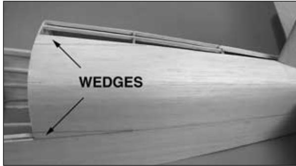
□ □ 10. Trim another 1/16" x 3" x 24" [1.6 x 76.2 x 610mm] balsa sheet to fit between the bottom turtle deck sheet and the center of the top, **center** stringer. Trim the aft end of the sheet so it fits the fin and ends at former F10A. Glue the sheet in position. Make a *wedge* from a 1/16" [1.6mm] leftover piece of balsa to fit between the two turtle deck sheets in the front.
