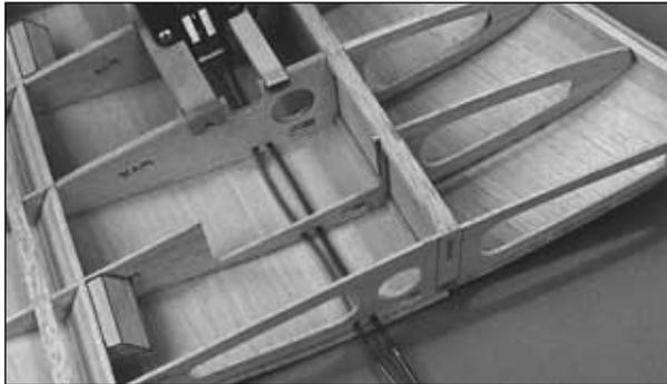
□ □ R13. Now is a convenient time to plan your air line routing. If you haven't already done so, drill or cut holes in the ribs to guide the air lines. A 5/32" [4mm] brass tube sharpened at one end makes a great *drill* to cut holes through the ribs. Do not install the air lines at this time.
