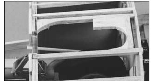
❑ 1. If you're installing retracts, turn the fuselage over and build a small *framework* from leftover balsa to support the sheeting around the nose wheel cutout.
