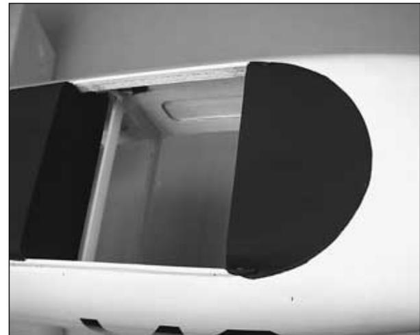
❑ 6. Fit and glue a die-cut 1/8" ply **instrument panel** in place where shown on the plans. Cut a piece from a manila file folder, using the pattern on the plan, to fill the area between the front of the fuselage and the instrument panel. Paint the material flat black after it is glued into place.
