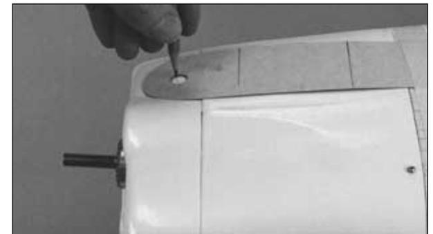
❑ 12. Replace the cowl on the fuselage and hold it in place with just a couple of the screws. Transfer the hole in the template to the cowl.
