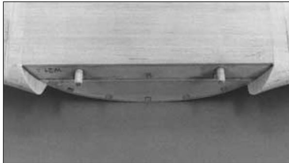
❑ ❑ 5. Remove the wing and sand the wing fairing block to match the shape of the **top** of the wing. The fairing block extends below the bottom sheeting, so blend it to the belly pan and the bottom of the wing with filler. Shape and fit the other fairing block the same way.
