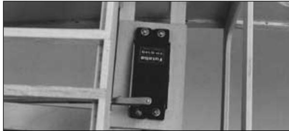
□ F12. Securely glue the nose steering servo tray to the servo rails. Make sure your servo is centered, and tighten up the 4-40 jam nut on the clevis with a drop of thread lock for extra security. File **small** flat spots in the nose gear to securely hold the set screws.
