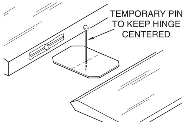
5. Join the elevators to the stab with the hinges. If necessary, insert a pin in the center of the hinges to keep them centered in the elevator and stab. Make sure there is approximately a 1/64" [0.4mm] gap between the elevators and the stab so you do not glue them together.
