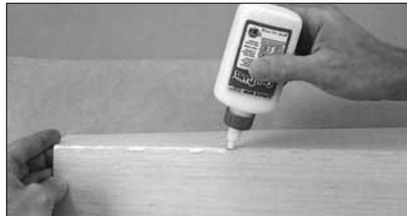
**C.** Place waxed paper on your workbench. Flip the sheets over and apply a bead of aliphatic resin (*wood workers glue* such as Great Planes Pro™) between the seams. Immediately proceed to the next step.
