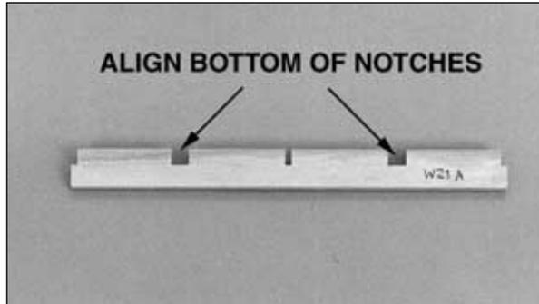
□ 5. Glue the die-cut 1/8" [3.2mm] plywood **leading edge doubler (W21)** to the die-cut 1/8" [3.2mm] plywood **center leading edge (W21A)** so the **bottoms** of the **notches** align. W21A is narrower than W21 so the top and bottom edges will be offset 1/16" [1.6mm].
