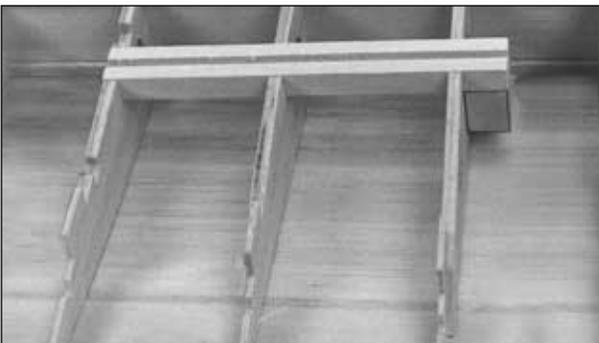
□ □ F14. Use 30-minute epoxy to glue the 1/2" x 3/4" x 6-3/4" [12.7 x 19 x 172mm] grooved hardwood **landing gear rail** in the notches of the ribs and rib doublers with the groove visible, as shown in the photo. At the same time, glue the 3/4" x 3/4" x 1" [19 x 19 x 25.4mm] maple **torque block** to rib doubler W4G and the top of the landing gear rail.
