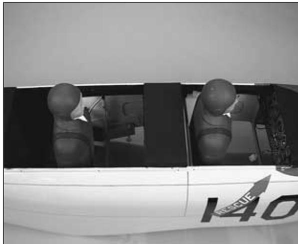
❑ 8. Remove the top of former F5 to make room for your pilots. We used 1/4 scale Williams Brothers pilots (the 1/5 scale pilots were undersize) and glued and shaped some balsa to the bottom of the pilot so it would extend lower into the fuselage. The pilots are glued to some 1/4" x 3/8" [6.4 x 9.3 mm] basswood sticks.
