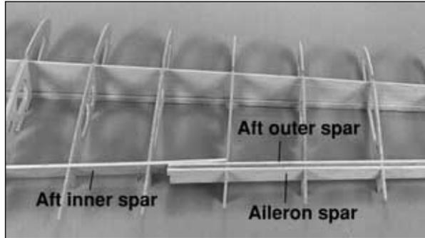
□ □ 5. Test fit the die-cut 1/8" [3.2mm] balsa **aft outer spar (W16)** and the die-cut 1/8" [3.2mm] balsa **aileron spar (W17)** into the notches of ribs W9 through W14. If necessary, bevel the notches in the spars and ribs the same way you did in the previous step.
