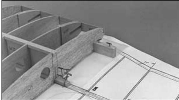
❑ 2. Make sure the center section accurately aligns with the plan. If necessary, pin two more balsa blocks to the building board near the fronts of the ribs.
