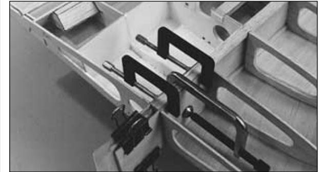
❑ 9. Insert two approximately 2" x 2" [50.8mm] pieces of waxed paper between the dihedral braces where they protrude from the right panel, then insert a piece of 1/8" [3.2mm] balsa between the two pieces of waxed paper. Clamp the outer 1/16" [1.6mm] ply dihedral braces to the inner 1/8" [3.2mm] ply dihedral braces.
