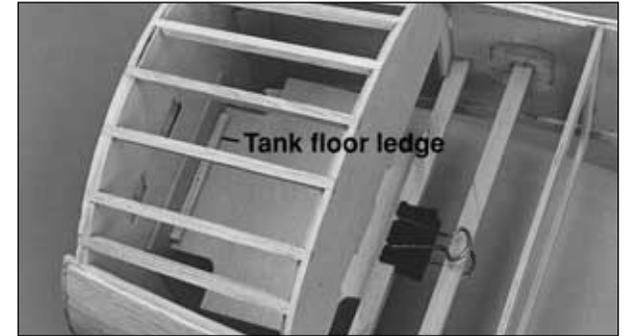
❑ 8. Temporarily clamp the die-cut 1/8" [3.2mm] plywood **tank floor** to the forward servo rail so it is centered on the back of the firewall doubler. Turn the fuselage over and push the tank floor up until it contacts the edge of the bottom blind nuts. Glue a 3/16" x 3/16" x 3" [4.8 x 4.8 x 76.2mm] balsa stick to the back of the firewall under the tank floor to serve as a **forward tank floor ledge**. Do not glue the tank floor to the ledge until instructed to do so.
