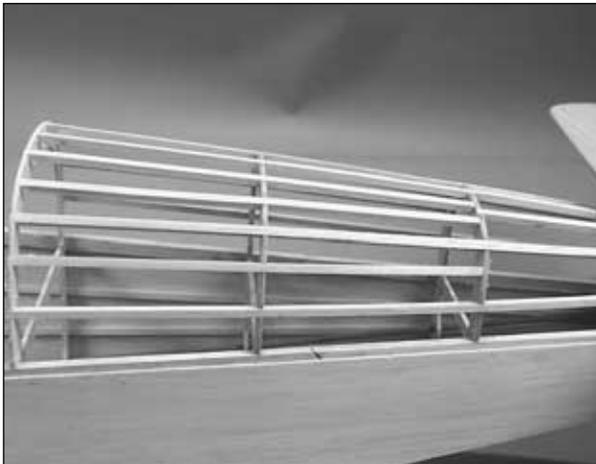
❑ 2. Cut the **turtle deck stringers** from seven 3/16” x 3/16” x 30” [4.8 x 4.8 x 762mm] balsa sticks. Glue the stringers into the notches of the formers as shown on the fuselage plan and in the photo. Note the arrangement of the stringers at F9A.
