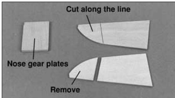
❑ F1. Draw a line connecting the punch marks on both die-cut 1/8" [3.2mm] plywood **nose landing**
