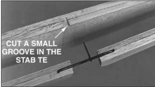
❑ 51. Cut a small groove in the TE of the stab so the **horn** on the elevator joiner will not bind against the stab when the elevator deflects downward. Test fit the elevators to the stab, with the elevator joiner in place, and make adjustments if necessary.
