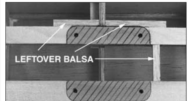
❑ 13. If you're installing retracts, glue leftover 3/16" or 1/4" [4.8 or 6.4mm] balsa to the front of the forward landing gear rail and between the rails to support the sheeting. Use a ballpoint pen or a pencil
