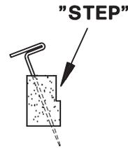
❑ 2. Pin the stringers over their location on the plan so the **step** is on the bottom and faces the outside of the fuselage. The front end of the stringers should align with the **dashed lines** near the front and extend past the firewall by 1/8" [3.2mm]. Use plenty of T-pins to hold the stringers down so they conform to the curvature of the plan.
