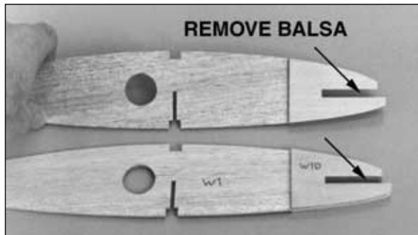
□ 7. Remove the balsa from both W1 ribs between the notches of the dowel doublers.
