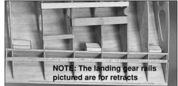
□ □ 19. Cut three 1-1/2" [38mm] long **flap hinge blocks** from the shaped 5/8" x 9" [15.9 x 229mm] balsa stock. Bevel one end of each hinge block so they fit the ribs, then glue them in the location shown on the plan. **See the cross section** on the wing plan to be sure you know the position and orientation of the blocks.
