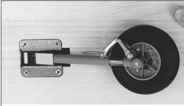
□ □ R1. Start by cutting and removing just enough sheeting to mount the landing gear to the rails.
