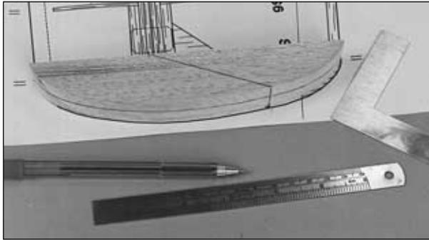
□ □ 41. Place the stab tip block over its location on the plan. Mark where the elevator tip meets the stab tip on both sides of the block.
