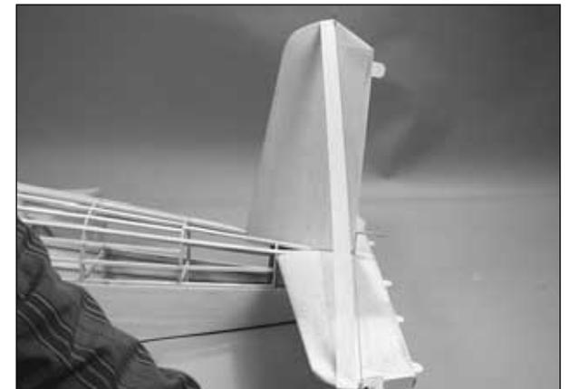
❑ 4. Mix some 30-minute epoxy. Glue the basswood stick into the fin making sure to put epoxy on the end of the stick that touches R2 inside the fin. Glue the fin and stick to the top of the stab and to former F10.
