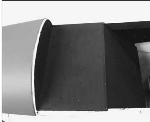
❑ 7. Use some leftover 3/32" [2.4mm] balsa sheeting to fill the rear cockpit area as shown on the plan and in the photo above. Paint the area black.
