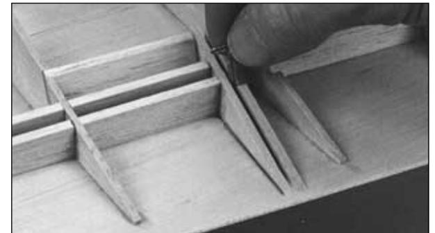
❑❑ 3. Stick a pin through the wing sheeting in a few places along the space between W8A and W9A, along the space between W2A and W2D, and along the space between W14A and W14. These pin points will indicate where to cut the sheeting to separate the ends of the flap and aileron from each other and the wing.
