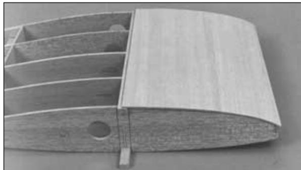
❑ 4. Sand the sheets so they are flat and smooth. Trim the forward skin so the aft edge aligns with the center of the top spar and the front extends past the LE (W21 and W21A) by approximately 1/8" [3.2mm]. If you find it necessary, wet the top of the forward top skin first, before gluing it to the center section of the wing. *You're an expert at sheeting now, so this should be easy.*
