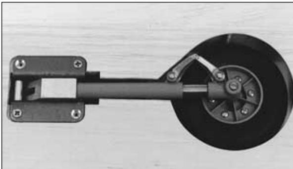
□ □ R2. Retract the gear so that the wheel lays on the wing sheeting and draw a rough outline of the wheel onto the sheeting. Cut the sheeting within the outline. Retract the wheel again and draw a more accurate outline. Cut the sheeting until the wheel fully retracts into the wheel well, leaving at least 1/8" [3.2mm] clearance between the wheel and the sheeting (in case you *tweak* your landing gear on one of those bumpy landings).
