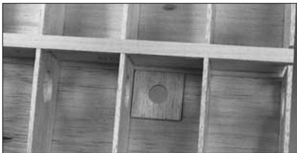
❑ 15. Glue a piece of leftover 3/32" [3.2mm] balsa to the center section sheeting aft of the spar (note the grain direction). Cut a 3/4" [19mm] hole through the sheeting at this location for the servo cords and air lines to exit the wing into the fuse.
