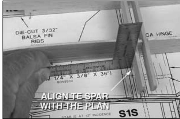
❑ 3. Use a small square to position the fin TE spar over the plan near rib R2. Align rib R2 over the plan and pin it to your building board. Use one T-pin near the front of the jig tab and one T-pin near the rear of the jig tab.
