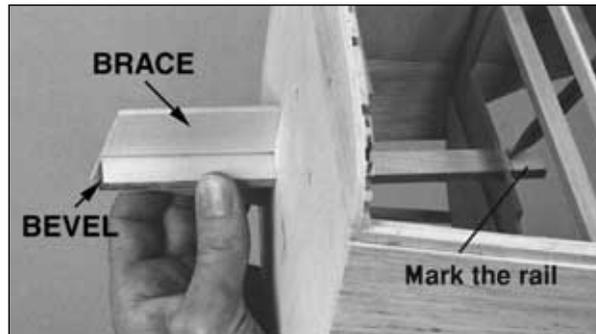
❑ F4. Cut a bevel on the end of the 1/4" x 9/16" x 9" [6.4 x 14.3 x 228.6mm] plywood **landing gear rails** to match the angle on the end of the braces. Test fit a rail through the right side of the firewall and in the notch in former F2. Position the right brace and align the front of the rail with the front of the brace. Mark the rail 1/8" [3.2mm] aft of former F2. Remove the rail and cut it at the mark. Mark the other rail in the same manner.
