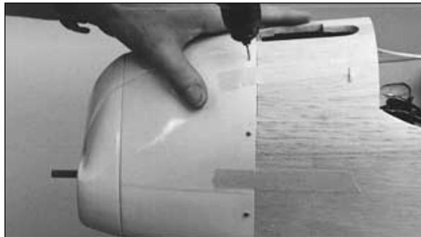
❑ 7. Securely tape the cowl to the fuselage. Using the marks as a guide, drill 1/16" [1.6mm] holes through the cowl and the cowl mount blocks 1/4" [6.4mm] in front of the aft edge of the cowl.
