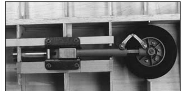
❑ ❑ R12. Drill holes in the rails and mount your landing gear. Use the screws included with your landing gear. Remove the landing gear and reinforce the holes with a few drops of thin CA. When the CA has cured, reinstall the landing gear. **Hint:** Countersink the holes in the landing gear for #6 x 1/2" [12.7mm] flat head screws.
