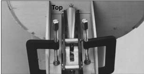
❑ R5. Use small clamps to hold the nose gear to the rails so the pivot point (on the Robart 631's) aligns with the marks you made on the top of the rails. Mark the locations of the mounting holes on the landing gear rails.
