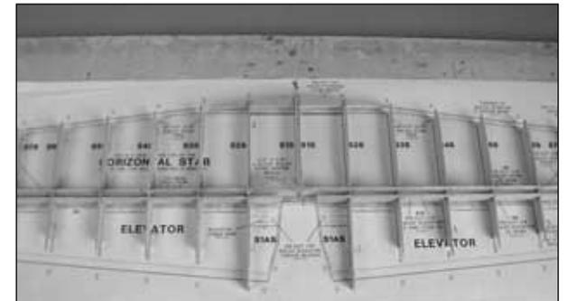
❑ 7. Add both die-cut 1/8" [3.2mm] balsa **elevator LE spars (S8)** to the assembly.
