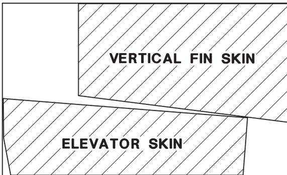
❑ 4. Cut the **stab, elevator, vertical fin and rudder skin templates** from the plan. Use a straightedge and ballpoint pen to mark their outline onto the 9" x 15" [229 x 381mm] planks (do not use a felt-tip pen). The templates are slightly oversize to allow slight variances in construction. Note the **grain direction**.
