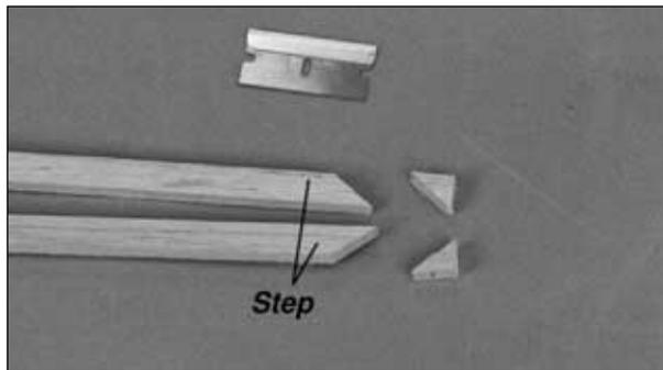
❑ 1. Cut a 45 degree angle at the aft end of two 1/4" x 3/8" x 36" [6.4 x 9.6 x 914mm] stepped balsa **side stringers** so you can *splice* them onto another stringer later.
