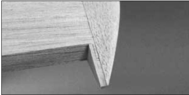
□ □ 2. Sand the sheeting and the *rib stubs* on the wing even with the TE. Glue a piece of leftover 3/32" [2.4mm] balsa to the wing tip rib. Sand it to the shape of the wing.
