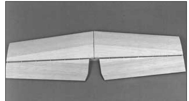
❑ 28. Glue the elevator skins to the bottom of the elevators so the trailing edges align.
