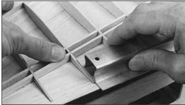
❑ 23. Use a bar sander and 150-grit sandpaper to bevel the trailing edge of the top elevator skin so it will accommodate the bottom skin. While you sand, apply pressure only to the sheeting and use the ribs to set your sander at the correct angle. Do not bevel the trailing edge to a *sharp edge* but leave about 1/32" [0.8mm] *squared off*. **Hint:** Support the TE with the edge of your workbench or a platform while you sand.
