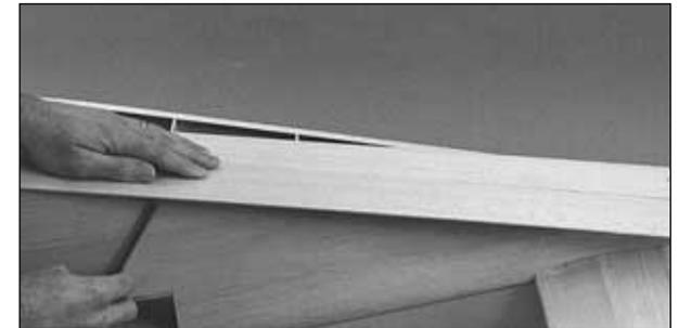
❑ 3. True both edges of another 3/16" x 3" x 30" [2.4 x 76.2 x 762mm] balsa sheet. Position the sheet on the bottom of the fuselage next to the center sheet. Use a ballpoint pen to mark the side of the fuselage onto the sheet. Cut the sheet along the line you drew. Do the same with the remainder of the sheet on the other side of the fuselage.
