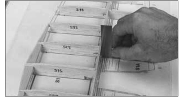
❑ 4. Use a small square to align the stab TE spar at rib S2S over the plan. Pin rib S2S over its location on the plan with a T-pin about 1/4" in front of the TE spar. **Note:** The above photo shows S1S in place, but it is not installed until step 11.
