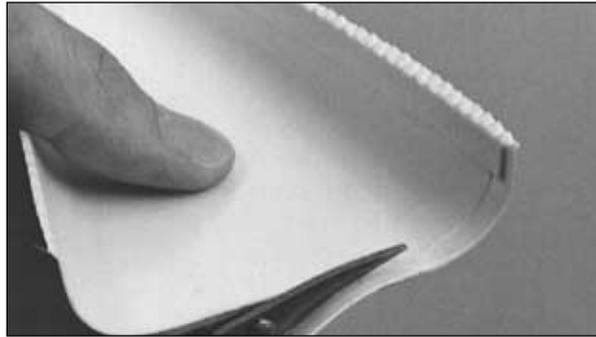
❑ 3. Cut both formed ABS **tail cone halves** along the cutlines. The cutlines can be most easily seen from the inside. We highly recommend a pair of Hobbico curved tip Canopy Scissors (HCAR0667) because you can cut straight lines or small tight curves easily and accurately. You could also use a small pair of regular scissors or **score** the plastic along the cutlines with a hobby knife and flex the plastic until the excess breaks free.
