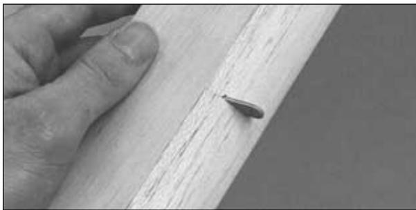
□ □ 10. Drill a 1/16" [1.6mm] hole through the punch mark in the front of the flap horn for the clevis. Add a few drops of thin CA to the hole. After the CA hardens redrill the hole. Remove the flap LE you tack glued on. Insert the flap horn into the flap and securely glue it in place. Permanently glue the flap LE to the flap.
