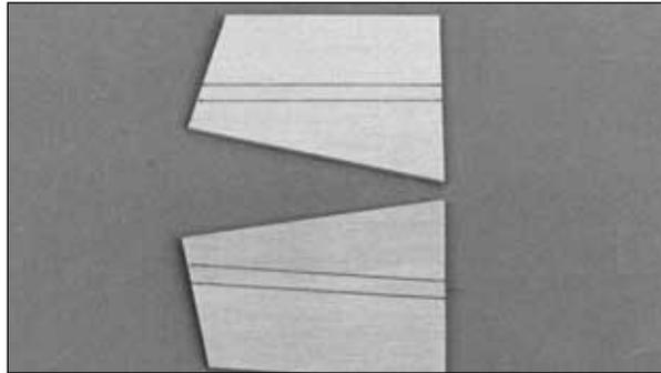
❑ F2. Place the braces over the **nose gear detail** on the plan. Mark the location of the 1/4" [6.4mm] plywood landing gear rails onto the braces.
