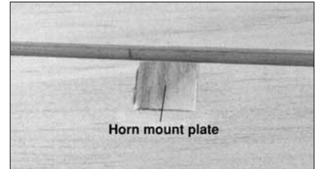
□ □ 1. Cut a 1/8" [3.2mm] deep notch in the aileron for the die-cut 1/8" [3.2mm] plywood **aileron horn mounting plate** where shown on the plan. Glue the horn mounting plate to the aileron and sand it to match the leading edge.
