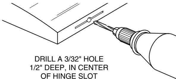
1. Drill a 3/32" [2.4mm] hole 1/2" [12.7mm] deep in the center of the hinge slots on the stab and elevators. A high speed Dremel Tool® with a cutting
