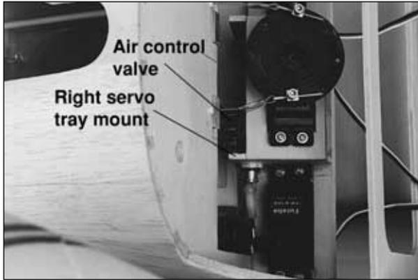
❑ 5. Mount your air control valve and servo. On our prototype we mounted the air control valve to the right nose steering servo tray. Mount yours the same way or find an alternate location. Mount the servo to two rails made from leftover 1/4" x 3/8" [6.4 x 9.6mm] basswood.
