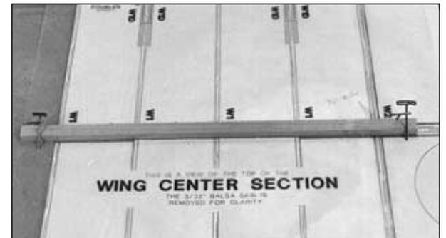
□ 9. Cut one 11" [279mm] long piece for the **bottom center spar** and one 9-1/4" [235mm] long piece for the **top center spar** from a 1/4" x 3/8" x 24" [6.4 x 9.6 x 610mm] basswood stick. Pin only the ends of the 11" bottom center spar to your building board over its location on the plan. Do not stick the T-pins through the basswood spar but insert them in a crossed fashion over the spar to hold it to your building board.
