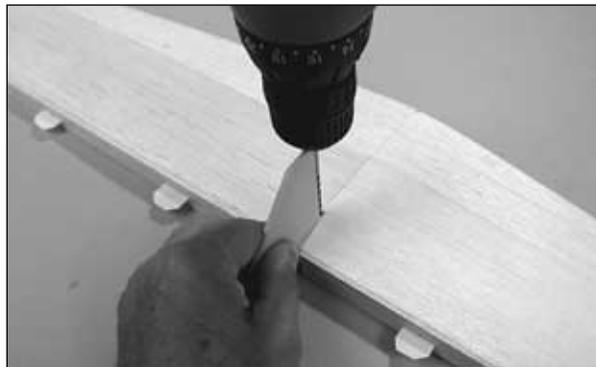
❑ 6. Mark the **center** of the stab 1-1/8" [28.6mm] from the TE. Drill a 1/8" [3.2mm] hole through the center of the stab at the mark. Use the die-cut 1/8" [3.2mm] ply **90 degree gauge** as a guide to keep the
