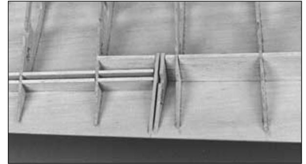
❑❑ 2. Glue the die-cut 3/32" [2.4mm] balsa **flap ribs W2A** and **W8A** and **aileron ribs W9A** and **W14A** to the wing where shown on the plan. Note that W8A and W9A are perpendicular to the aileron spar W17. **Hint:** Temporarily place a *shim* made from 1/16" [1.6mm] leftover plywood between the ribs for perfect alignment.
