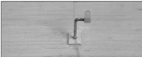
❑ 10. Make a 1/2" x 1/2" [12.7 x 12.7mm] **bearing block** from some leftover 1/8" [3.2mm] ply. Drill a 1/8" [3.2mm] hole in the center of the block and install it on the torque rod on the **bottom** of the stab. Glue it in place with medium CA, being careful not to get any on the torque rod. Make sure that the nylon swivel horn has been installed on the threaded end of the torque rod, with the tab pointing towards the front of the stab.
