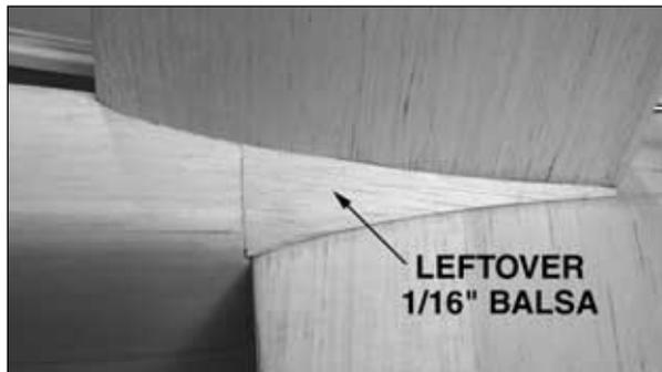
□ □ 11. Fill the space between the fin and the stab with a leftover piece of 1/16" [1.6mm] balsa.
