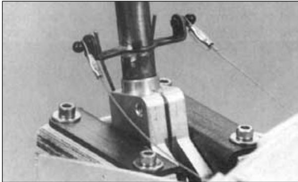
❑ R2. Install a 0-80 threaded ball link ball (not included) onto the arm on both sides of the nose wheel strut with a 0-80 nut. Connect the other end of both cables to the threaded ball links with the swages. Tighten the loop in the cable just enough so it will not come off the ball. Crimp the swages. Temporarily hook up the steering servo to your radio system and test the movement. Adjust the tension on the cables or make other adjustments if needed.
