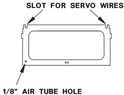
❑ 6. If you plan to install the Top Flite Beechcraft T34B Scale Cockpit Kit (TOPQ8413), drill holes and cut slots in the formers for routing the air lines and servo wires between the fuse sides and the cockpit interior in formers **F3**, **F4** and **F5**.
