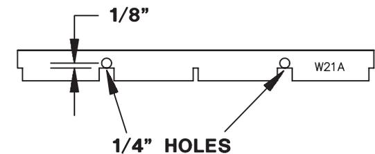
❑ 9. Drill 1/4" [6.4mm] holes through the LE of the center section (W21 and W21A) where shown on the sketch. Slightly round one end of both 1/4" x 2-1/2" [6.4 x 63.5mm] **wing dowels**. Test fit, then glue the wing dowels into the center section with 30-minute epoxy. The rounded end should point out the front of the LE.
