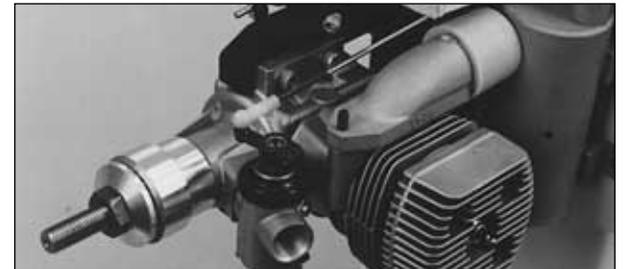
*This is the throttle servo location for retractable gear.*
