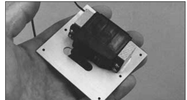
□ □ 4. Mount each servo to two 5/16" x 3/4" x 7/8" [7.9 x 19 x 22.2mm] **servo mount blocks** with the screws, grommets and eyelets included with your servos. Remove the screws, harden the screw holes with some thin CA and then reinstall the servo. Be sure that the servo is aligned so that the servo arm is in the center of the cutout.
