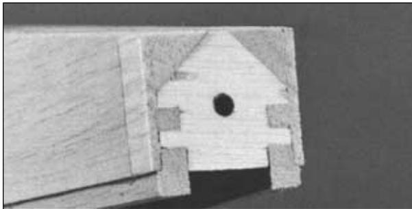
❑ 11. Trim, then sand the fuselage side sheeting and stringers that extend aft of former F11 so they are flush.
