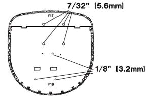
❑ 6. Drill the correct size holes through the punch marks on the front of the firewall as shown in the sketches above. Tightly hold a **thick** block of wood on the back so the drill does not split the wood when it comes through.
