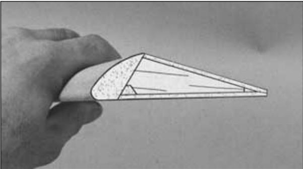
□ □ 9. Cut the **flap root and tip end templates** from the plan. Glue them to the ends of the flap with rubber cement or spray adhesive. Use the templates as a guide to shape the flap LE with a razor plane or a hobby carving knife followed by a bar sander.
