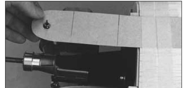
❑ 11. Remove the cowl and make a template out of thin cardboard to locate the needle valve. Tape it to the fuselage.
