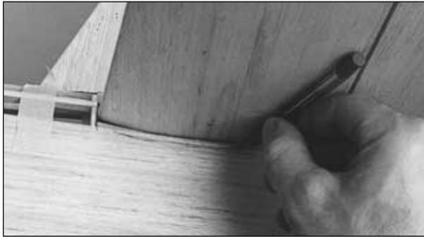
□ □ 6. Use a ballpoint pen to mark the bottom of the stab onto the sheet. Remove the sheet and cut along the line you marked.
