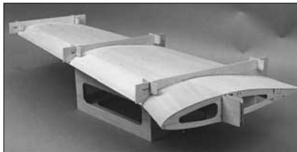
❑ 4. Glue the die-cut 1/8" [3.2mm] balsa **feet** to the cradles. Apply one drop of thick or medium CA near the
