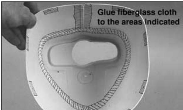
❑ 15. Make sure you have thoroughly sanded the inside seams of the cowl. Use 30-minute epoxy to glue 1" [25.4mm] wide **fiberglass cloth** over all the seams inside the cowl. Add 1" [25.4mm] squares of glass cloth inside of the cowl over the holes for the cowl mount screws. Redrill the holes after the epoxy cures.
