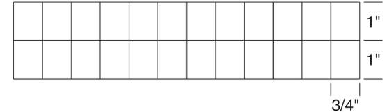
❑ 37. Cut six **hinges** from the 2" x 9" [51 x 229mm] **CA hinge strip** as shown in the sketch. Snip the corners off the hinges so they go into the slots easier. Temporarily join both elevators to the stab with the hinges. If necessary, adjust the hinge slots so the elevators and stab align.
