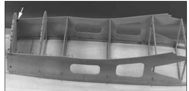
❑ 7. Test fit, then glue the die-cut 1/8" [3.2mm] plywood **fuse side doublers** to formers **F2** through **F6** only and to the side stringers. **Do not** glue the doublers to the firewall until the next step. You may have to reposition some of your T-pins so they do not interfere with the side doublers. Use your 90 degree triangle to hold the formers vertical while you glue the doublers to them.
