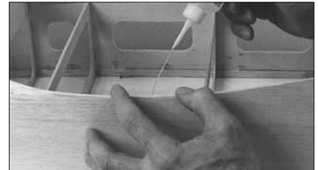
❑ ❻ 6. A little section at a time, carefully pry the fuse side from the fuse side doubler and apply thin or medium CA between the two. Quickly press them together. Do this until the fuse side is thoroughly glued to the side doubler.
