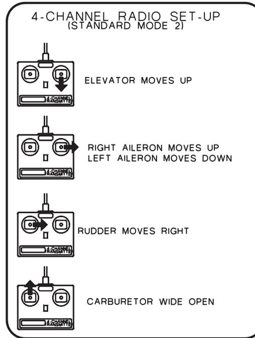
❑ 12. Adjust your pushrod hookups and set up your radio to provide the control surface movements as follows.
