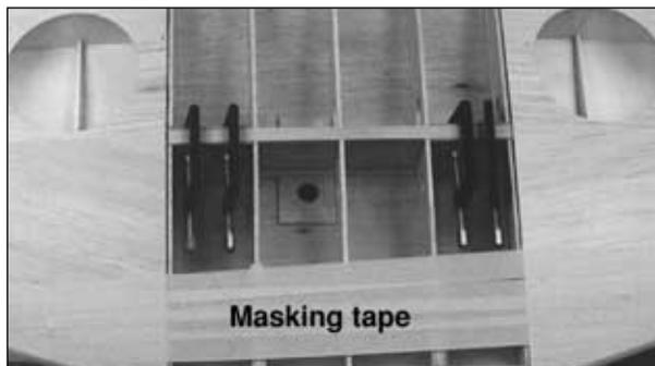
□ 1. Remove the flaps. Test fit both outer panels to the center section. Make small adjustments if necessary to minimize any gaps you see. *Test fit* your clamps to make sure you have enough of them and to make sure you know where you are going to place the clamps when you actually glue the wing together.
