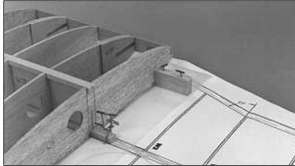
❑ 2. Make sure the center section accurately aligns with the plan. If necessary, pin two more balsa blocks to the building board near the fronts of the ribs.
