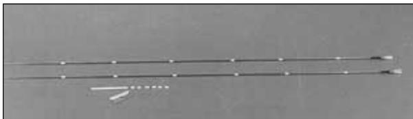
❑ 11. Cut 7" [177.8mm] from the non-threaded end of a .074" x 36" [1.9 x 916mm] **pushrod wire**. Clean residual oil from the wire with a cloth dampened with alcohol or other solvent. Cut six 1/4" [6.4mm] long
