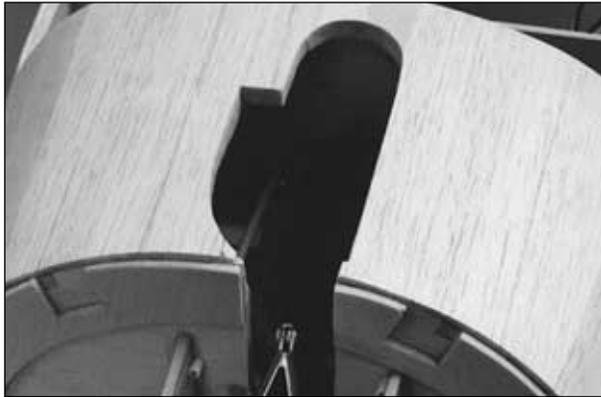
❑ 3. Use leftover 3/32" [2.4mm] balsa sheet to sheet the bottom forward fuse, between the firewall and F2. Cut the wheel well for the nose wheel and strut if you are installing retracts.
