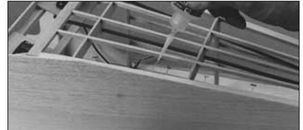
❑ ❑ 5. Apply a bead of medium CA to the *step* portion of the stepped balsa side stringer from the firewall to former F6. Working quickly, position the side sheet on the ledge of the side stringer and press it into position where you have applied the glue. After the CA dries apply thin CA to the side stringer and side sheet aft of former F6 from inside the fuse. A long CA applicator tip, such as the Hobbico applicator tip (HCAR3780), helps you apply the CA just where you need it.
