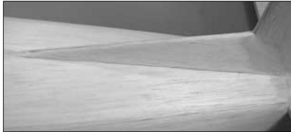
❑ 4. Apply Hobbylite™ filler to the dorsal fin and fin filler sheet to blend them to the fin. Apply filler to the front of the dorsal fin to complete the taper and blend it to the turtle deck. Do not apply all the filler in one application but build up thin layers, allowing each layer to fully dry before you apply the next. Sand the filler, blending the dorsal fin, fin filler and fin into one smooth contour.
