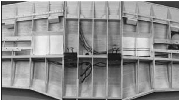
*We've temporarily joined the wing panels and installed the air lines and servo leads in the right wing panel to mock-up the installation to give you an idea of how to route them later. If you wish, you could test your installation now to make sure your setup will work.*
