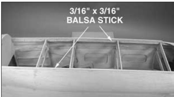
❑ 1. Cut two 3/16" x 3/16" x 30" [4.8 x 4.8 x 762mm] balsa sticks to a length of 21" [533.4mm] and glue one to each canopy base, along the inside edge. See the "cross section at former F5" view on the plan.
