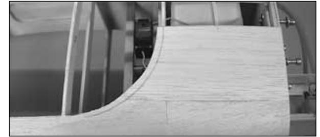
❑ 11. Use a short piece of 3/32" [2.4mm] balsa sheet and glue it in place on the top of the fuselage from the firewall to F2. The sheet should be trimmed at the center of the center stringer. Note that we traced the shape of the canopy onto the sheeting.
