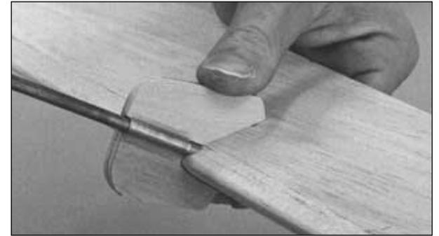
□ □ 14. Use the **flap hinge drill guide** to drill holes in the flap the same way you did for the wing.
