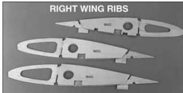
□ F7. Prepare a set of **right** wing ribs by using 30-minute epoxy to glue the die-cut 1/8" [3.2mm] plywood **fixed landing gear rib doublers W4G, W5G and W6G** to the die-cut 3/32" [2.4mm] balsa **ribs W4, W5 and W6 exactly** as shown in the photo. Make sure the doublers are on the side of the ribs as shown in the photo.
