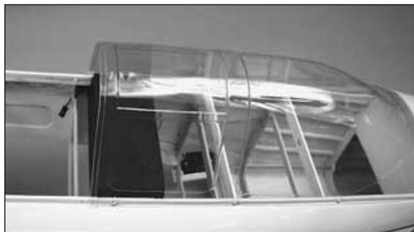
❑ 3. Cut the rear canopy out on the cut lines and fit the canopy into place on the fuselage. We held the rear canopy in place with eight #2 x 3/8" [9.5mm] sheet metal screws.
