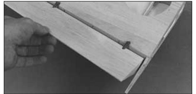
□ □ 15. Cut 1/4" [6.4mm] off the end of the outermost hinge point that fits into the flap. Test fit the flaps to the wing with the hinge points. Adjust the position (depth) of the hinges until the flap aligns with the wing the same way it was before you cut it loose. Make adjustments until the flap fits the wing and freely moves about its range of motion. Strive for a good fit where the top of the flap meets the top of the wing.
