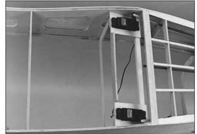
❑ 5. Position the rail and the servo trays so the servo arms align with the pushrods. Glue the rail and servo trays to former F5 and the fuse sides in this position. Drill 1/16" [1.6mm] holes in the servo trays and then harden the holes with some thin CA. Mount the servos with the screws, grommets and eyelets that came with your radio.
