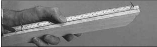
❑ 34. Use two T-pins, placed in the **center** of the leading edge of one of the elevators near the ends, to align a straightedge and draw a centerline with a ballpoint pen.
