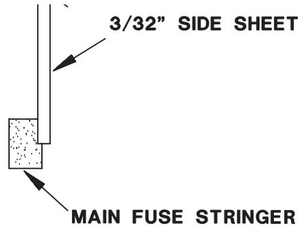
❑ ❑ 2. True one edge of the fuse side sheet. Hold the side sheet on the right fuse side with the front of the sheet about 1/4" [6.4mm] past the firewall. The sheet should rest on the edge of the step in the stepped balsa side stringers. Mark the wing saddle and corner stringer on the sheet. Trim the sheet about 3/16" [4.8mm] outside of the lines.
