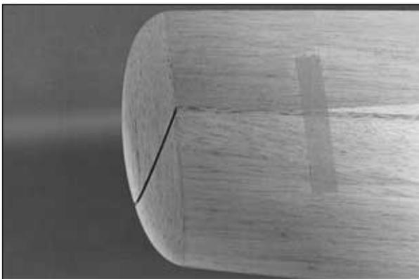
□ □ 44. Use a razor plane or a hobby carving knife, followed by sanding to **carefully** shape the elevator and stab tip. Inspect your progress frequently. Use the centerlines as a guide and the plan as a reference so you know what the curve of the tip should look like.
