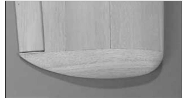
□ 1. Locate the 1-1/2" x 1-9/16" x 9" [38 x 39.7 x 228.6mm] shaped balsa **wing tips**. Check the shape of the tips against the plan and sand as needed to fit.
