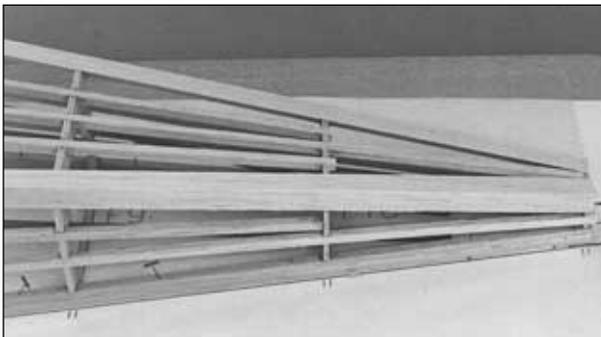
❑ 10. Glue the 3/16" x 1/2" x 10" [4.8 x 12.7 x 254mm] balsa bottom **fuse sheeting support** in position. Sand the ends even with the fuse side doublers. Cut and fit, but **do not glue** the aft bottom fuse stringers from seven 3/16" x 3/16" x 30" [4.8 x 4.8 x 762mm] balsa sticks to fit in the notches of the formers as shown on the plan and in the photo. Save the leftover pieces. The three bottom stringers extend to the sheeting support. You can see the stringers in the photo at step 5 page 37.
