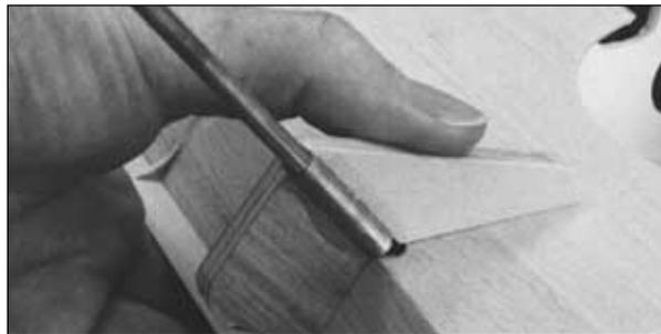
□ □ 12. Position the **wing flap hinge drill guide** on the wing over each hinge block (you marked them before you sheeted the bottom of the wing) and drill 3/16" [4.8mm] holes 1-1/8" [28.6mm] deep for the Hinge Points. **Hint:** Instead of using a drill bit, use a piece of 3/16" brass tube sharpened at one end to drill holes with clean edges.
