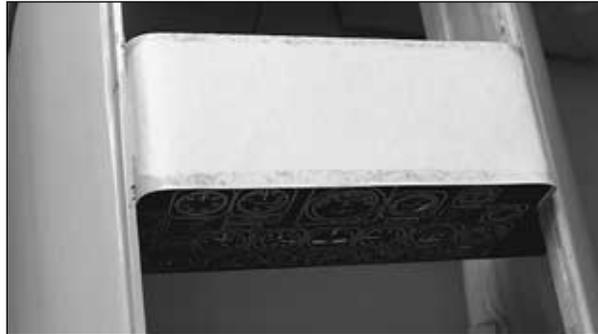
❑ 2. Fit and glue two die-cut 1/8" ply **instrument panels** in place where shown on the plans. Cut a piece from a manila file folder to fill the area between the two instrument panels. Paint the material flat black after it is glued into place.
