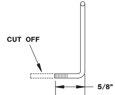
❑ 7. Cut the threaded end of the **rudder torque rod** so the threads extend 5/8" [15.9mm] as in the sketch. Tap threads in the nylon **swivel horn** with a 6-32 tap. Thread it onto the rudder torque rod until it is even with the end.
