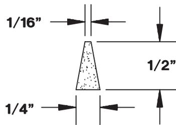
❑ 2. Cut the 15" [381mm] tapered balsa **dorsal fin LE** to the shape shown on the plan. Glue the dorsal fin LE to the fin LE and the dorsal fin base.
