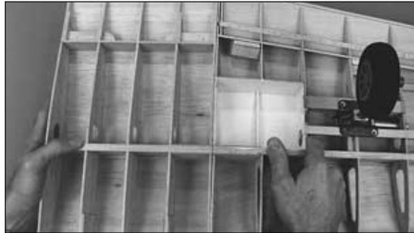
❑ 5. Temporarily join the center section to the right wing panel with the dihedral braces to make sure everything fits. Make adjustments where needed so the center section fully contacts the right panel. Separate the wing sections and remove the dihedral braces.
