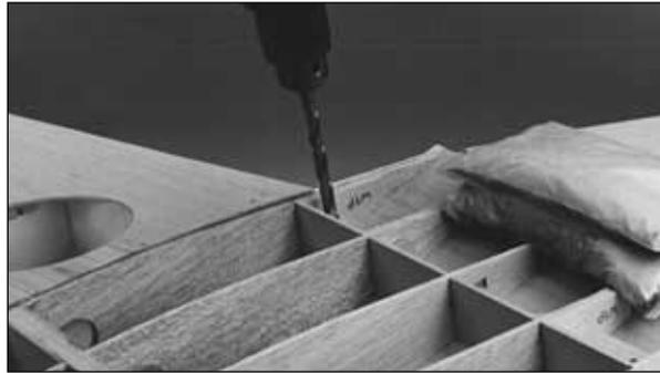
❑ 7. Drill through **only one** wing bolt plate, the top sheeting and the wing bolt block on one side of the wing with a #7 drill. Keep the drill bit perpendicular to the wing bolt plate as you drill so the head of the wing bolt will rest flat.
