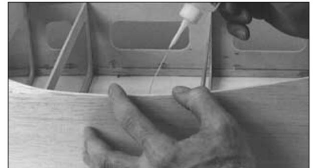
❑ ❑ 6. A little section at a time, carefully pry the fuse side from the fuse side doubler and apply thin or medium CA between the two. Quickly press them together. Do this until the fuse side is thoroughly glued to the side doubler.
