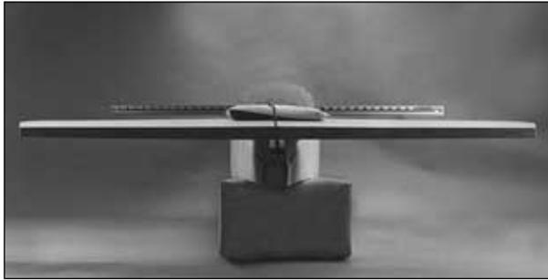
❑ 2. Stand behind the fuselage and view the stab and the straightedge to see if they align. If necessary, carefully sand one side of the stab saddle so the stab will align with the straightedge.
