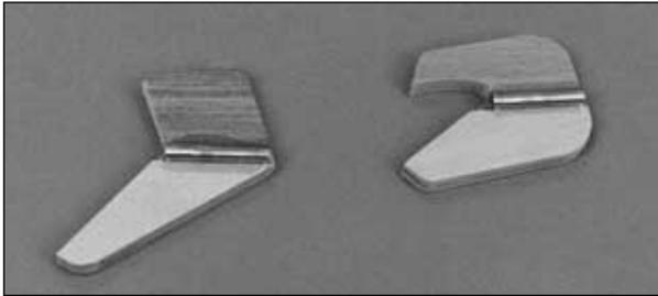
□ □ 11. Assemble the die-cut 1/8" [3.2mm] plywood **flap hinge drill guides** by gluing the pieces together as shown. **Optional:** Glue a piece of 7/32" [5.6mm] brass tubing (3/16" I.D. [4.8mm]) to the hinge drill guides to guide your drill even better.
