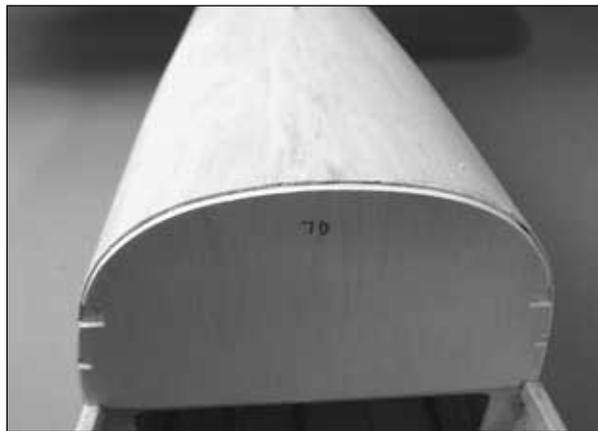
❑ 6. If you have not already sanded the turtle deck to shape then do so now. Remember, sand the 1/16" [1.6mm] balsa carefully. Fit the die-cut 1/8" [3.2mm] plywood former **F7D** to the front of F7A. Sand the edges of F7D so that there is a lip the thickness of the canopy. When you are satisfied with the fit, glue F7D to F7A.
