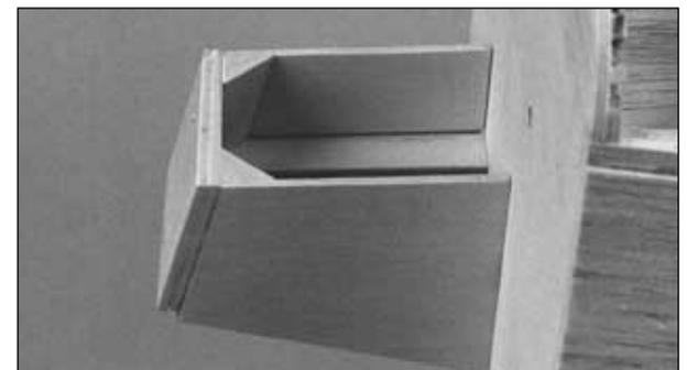
❑ F7. Position the nose gear plate on the front of the braces. Trim the rails so the blind nuts do not interfere. Use 30-minute epoxy to glue the nose gear plate to the rails and rail braces. Hold the plate in position with masking tape until the epoxy is fully cured. Add balsa triangle **braces** as shown on the plan cut from leftover fuse corner stringers. See the photo below at step 8.
