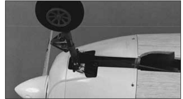
❑ 10. If you have fixed landing gear, cut a slot in the bottom of the cowl to clear the landing gear wire. If you have retractable landing gear, remove whatever material is necessary so the retractable nose strut and steering arm will clear the cowl.
