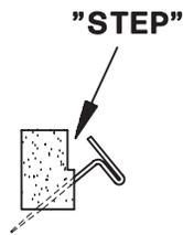
❑ 4. One at a time, remove the T-pins in the main side stringers aft of former F6. Replace them at an angle from the outside so they will not interfere with the side sheeting.
