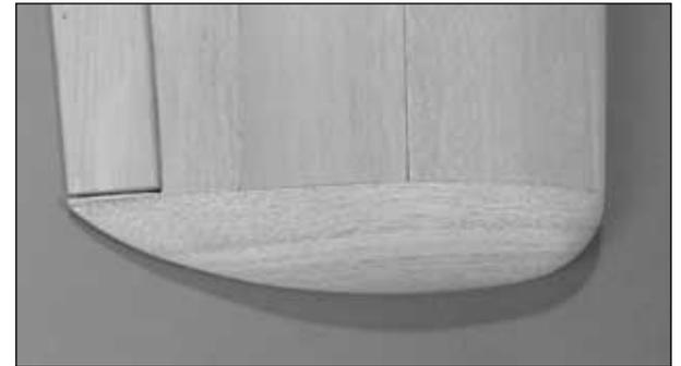
□ 1. Locate the 1-1/2" x 1-9/16" x 9" [38 x 39.7 x 228.6mm] shaped balsa **wing tips**. Check the shape of the tips against the plan and sand as needed to fit.
