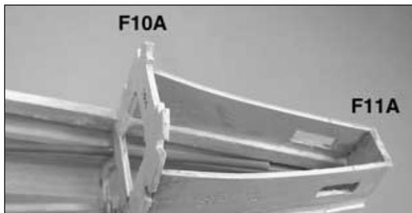
❑ 1. Glue the die-cut 1/8" [3.2mm] balsa **aft upper former F11A** to former F11.
