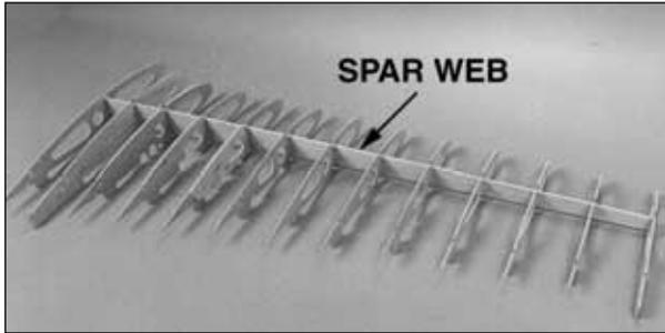
□ □ 2. Test fit ribs **W2 through W14** to the die-cut 1/8" [3.2mm] balsa **spar web (W15)**. If necessary, deepen the notches (in the ribs or in the spar web) so the ribs fit all the way into the spar web.
