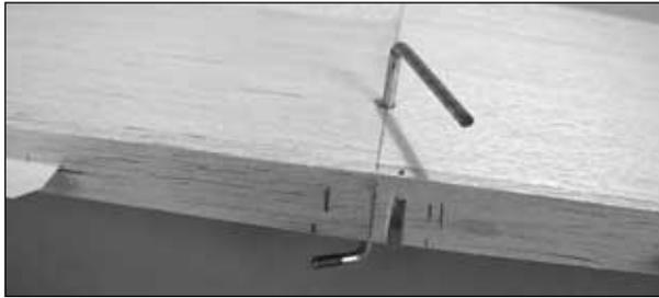
❑ 9. Insert the **rudder torque rod** into the hole in the stab from the bottom. Use a heavy duty pair of pliers to make the 90 degree bend in the torque rod. This bend is not hard to make if you hold the vertical portion of the torque rod with the pliers and then use your thumb, or another pair of pliers, to bend the torque rod over. Midway through the bend check that it is 90 degrees to the threaded end of the rod.
