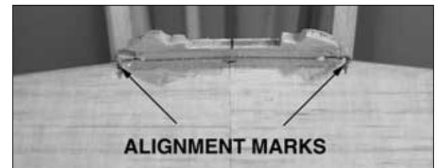
❑ 4. Mark the LE of the stab where it aligns with former F10A.
