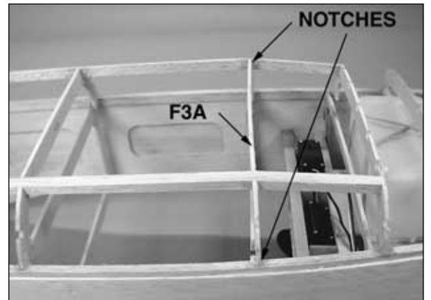
❑ 7. Make the **canopy base** from two 1/4" x 3/8" x 36" [6.4 x 9.5 x 915mm] balsa sticks. Cut them to fit between F2A to F7D. The sticks angle down between F2A and F3A so you will need to cut a notch in the stick at F3A. Glue the sticks in place, making sure they are firmly seated in the notches in the formers, especially at F7D.
