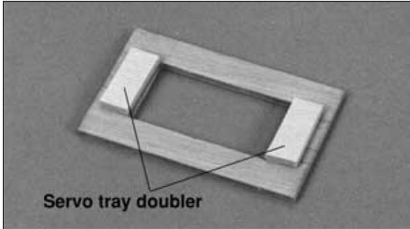
❑ 1. Glue the die-cut 1/8" [3.2mm] plywood **servo tray doublers** to the bottom of both die-cut 1/8" [3.2mm] plywood **forward servo trays**. Mount your throttle servo to one tray and your nose wheel steering servo to the other tray using the screws, grommets and eyelets that came with the servos.
