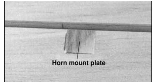
□ □ 1. Cut a 1/8" [3.2mm] deep notch in the aileron for the die-cut 1/8" [3.2mm] plywood **aileron horn mounting plate** where shown on the plan. Glue the horn mounting plate to the aileron and sand it to match the leading edge.
