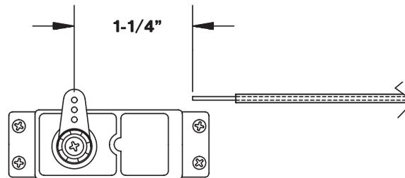
❑ 2. Place a servo arm on your rudder and elevator servos. With the servos centered and the rudder and
