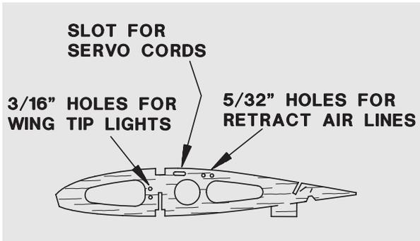
**R5.** Drill 5/32" [4mm] holes and cut slots at the locations suggested in the sketch in both sets of ribs W2, W3 and W4 for the retract air lines and servo leads. Make the slots large enough so the connectors on the ends of your servo leads will pass through. **Hint:** An appropriate size brass tube sharpened at one end cuts very clean holes.
