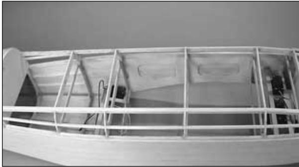
❑ 8. Cut **stringers** from 3/16" x 3/16" x 30" [4.8 x 4.8 x 762mm] balsa sticks to fit from the firewall to F7D and from the firewall to F2A. Use leftover sticks wherever possible. Glue the stringers into position.
