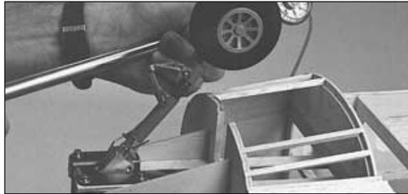
❑ R8. If you have your air pump and some quick disconnects handy, temporarily connect them to your nose gear air cylinder and actuate the nose gear with the air pump. This will give you a good indication of any problem areas that you can correct now.
