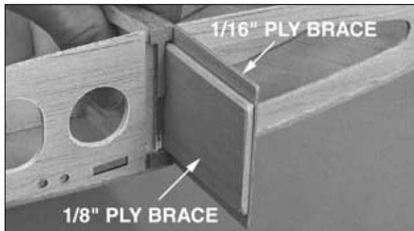
❑ 4. Test fit the die-cut 1/16" [1.6mm] plywood **dihedral braces W23** and the die-cut 1/8" [3.2mm]
