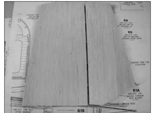
❑ 9. Glue the fin and rudder skin to the structure. The bottom of the fin skin should extend below rib R1 by approximately 1/4" [6.4mm] so you can trim it later. Make sure the trailing edge of the rudder meets the stoppers on the top of the jig tabs on ribs R2 and R6. **Note:** The rudder skin was cut wider than needed, to allow enough material to trim it to size now.
