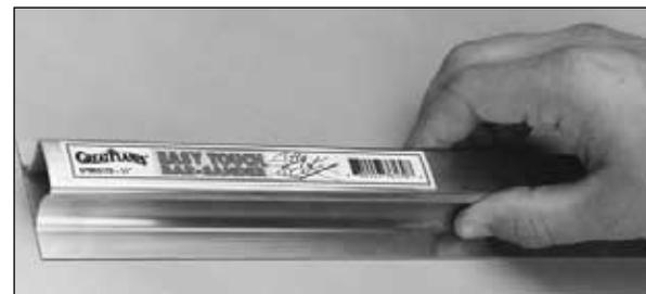
A flat, durable, easy to handle sanding tool is a necessity for building a well finished model. Great Planes makes a complete range of patented Easy-Touch Bar Sanders and replaceable Easy-Touch adhesive-backed sandpaper. While building the T-34B Mentor we used two 5-1/2" Bar Sanders and two 11" Bar Sanders equipped with 80-grit and 150-grit adhesive-backed sandpaper.
