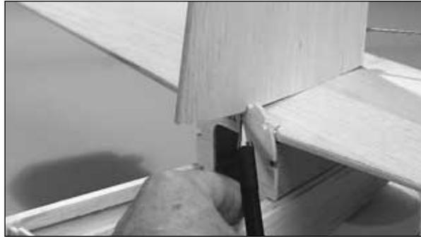
❑ 1. If you have not already done so, sand the sheeting on the bottom of the fin even with R1. Place the fin on the stab with the TE resting against the rudder torque rod. Mark the bottom of the fin at the front of fuselage former F10A.
