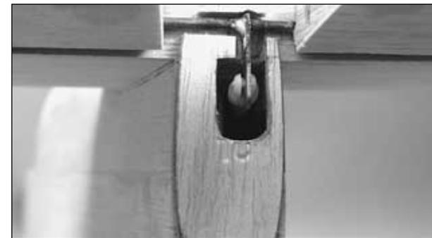
❑ 1. Fit the die-cut 1/8" balsa **tail cone former (F11TC)** on the aft end of the fuselage. Shape F11TC as needed to fit the end of the fuselage, allowing for the thickness of the ABS tail cone. Remove material as needed to clear the torque rods and pushrods. Glue F11TC into place. **There must be no possibility of binding here.**
