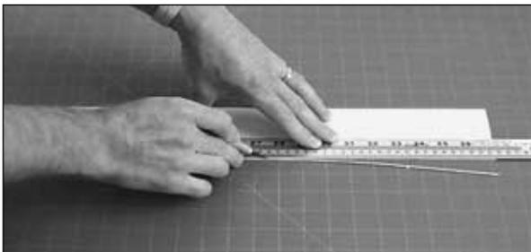
**A.** Use a straightedge and a sharp #11 blade to true the joining edges of the sheets. When you trim them, do not cut all the way through the first time but make several passes so you **slice** the wood instead of splitting it.
