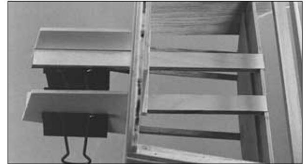
❑ F5. Use 30-minute epoxy to simultaneously glue the rails to the firewall and former F2, and the rail braces to the rails and the firewall. Make sure the front of the rails are even with the front of the braces.
