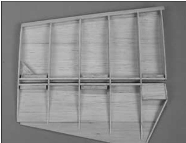
❑ 15. Glue the four die-cut 1/8" [3.2mm] balsa **rudder torque rod blocks** between ribs R1A and R2 in the rudder.
