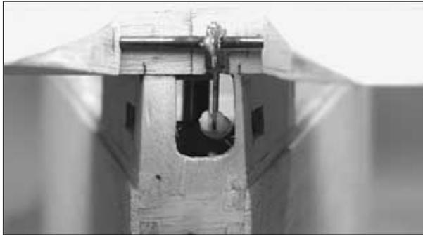
❑ 5. Test fit the rudder and elevator and temporarily hook up the pushrods. Make sure you can move the controls without any interference or binding. Make adjustments if necessary.
