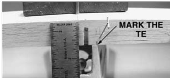
❑ 1. Align the TE of the stab with the center of former F11. Mark the TE of the stab above the stab saddles. Pin the stab TE to the stab saddle in this position.
