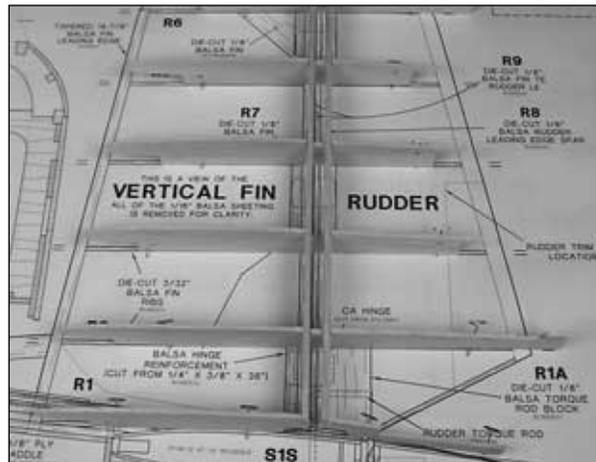
❑ 5. Pin rib **R1** in place and glue it to the spar. Cut the end off rib **R1A** at the embossed line and set the cut-off piece aside. Pin the remaining part of R1A in place and glue it to the rudder LE spar.
