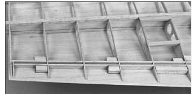
□ □ 21. Bevel the ends of all the aileron hinge blocks so they fit against the ribs as shown on the plan. Bevel the **tops** of the hinge blocks that fit in the aileron so they match the angle of the ribs. Glue the hinge blocks in the wing and aileron.
