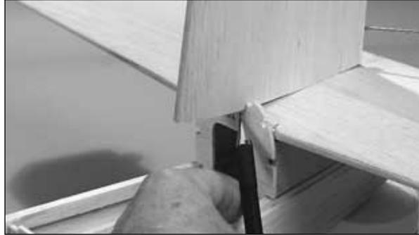
❑ 1. If you have not already done so, sand the sheeting on the bottom of the fin even with R1. Place the fin on the stab with the TE resting against the rudder torque rod. Mark the bottom of the fin at the front of fuselage former F10A.
