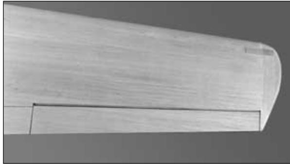
□ □ 6. Replace the flap onto the wing. Adjust the root of the aileron and the tip of the flap so there is approximately a 3/32" [2.4mm] gap between them.
