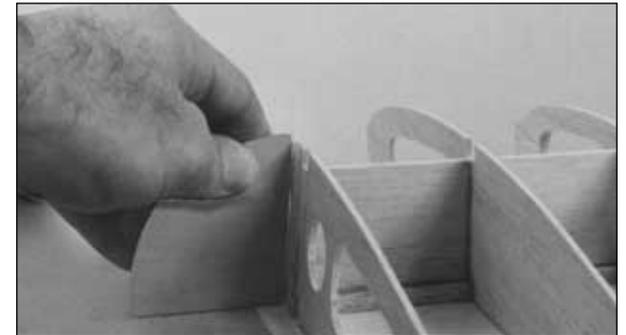
□ □ 9. Place rib W2 back onto the assembly. Align W2 with the dashed line depicting where it contacts the plan. Use the die-cut 1/8" [32.mm] plywood **dihedral gauge** to set W2 at the correct angle. Glue it to the bottom spar and the spar web. Glue W2 to the aft inner spar using the dihedral gauge to set it at the correct angle.
