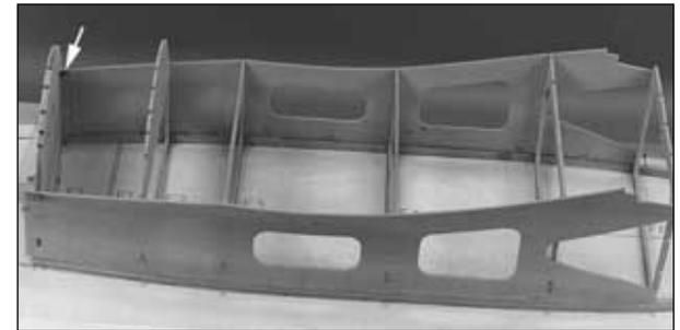
❑ 7. Test fit, then glue the die-cut 1/8" [3.2mm] plywood **fuselage side doublers** to formers **F2** through **F6** only and to the side stringers. **Do not** glue the doublers to the firewall until the next step. You may have to reposition some of your T-pins so they do not interfere with the side doublers. Use your 90 degree triangle to hold the formers vertical while you glue the doublers to them.
