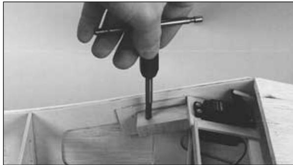
❑ 8. Remove the wing and tap threads into the wing bolt block with a 1/4-20 tap. Enlarge the hole in the wing bolt plate and the top sheeting with a round file or a 17/64" [6.8mm] drill. Replace the wing on the fuselage and bolt it down with the one 1/4" - 20 nylon wing bolt.
