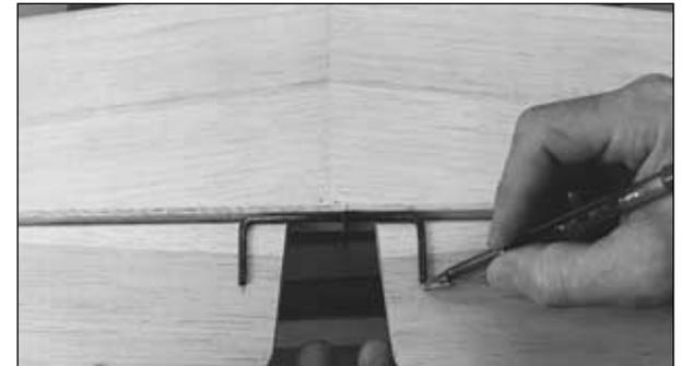
□ □ 49. Using the plan, accurately mark the location of the 1/8" [3.2mm] **elevator joiner wire and horn** (from now on referred to as just the **elevator joiner**) on the elevators.
