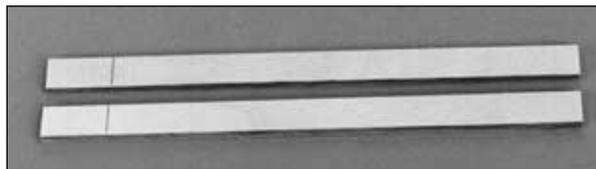
□ R1. If you're using the Robart 631 nose gear retract, mark a line 7-7/8" [200mm] from one end of both 1/4" x 9/16" x 9" [6.4 x 14.3 x 228.6mm] plywood **landing gear rails**. This will position the **pivot point** of the 631 nose gear 7-7/8" [200mm] from the aft edge of F2.
