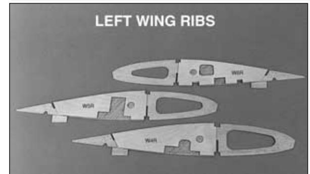
**R3.** Prepare a set of **left** wing ribs the same way but **use the photo above** to make sure you glue the doublers to the correct side of the ribs.
