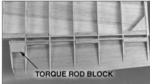
❑ 24. Glue four die-cut 1/8" [3.2mm] balsa **elevator torque rod blocks** between both sets of ribs S1AS and S2S.
