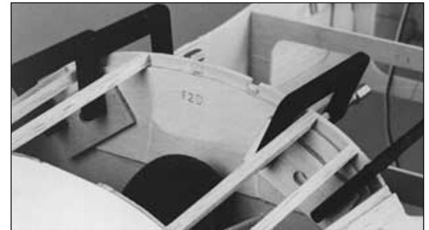
❑ 13. Remove the wing. Clamp the wing dowel plates to F2D with C-clamps. Wipe excess epoxy from the holes if any is present.
