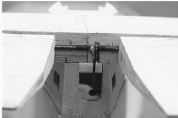
❑ 5. Use a hobby knife or a Multi-Pro™ with a sanding drum to cut F11A to clear the horn on the elevator joiner wire and the rudder torque rod.
