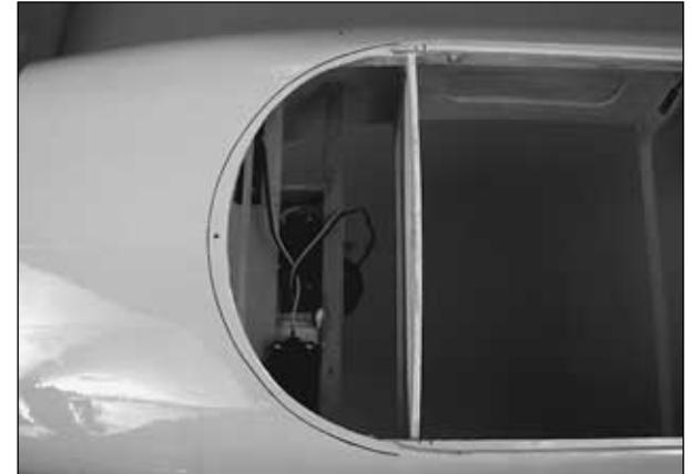
❑ 5. Trace the outline of the front canopy on the top of the fuselage with a fine point felt tip marker pen. Remove the front canopy from the fuselage.
