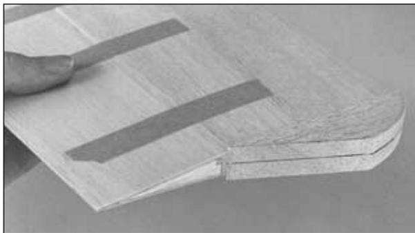
□ □ 43. Glue the **stab tip** to the stab. The sharp *point* of the stab tip should align with the TE of the stab. Glue the **elevator tip** to the elevator so it is 1/8" [3.2mm] aft of the LE and aligns with the stab tip (as shown in the sketch).
