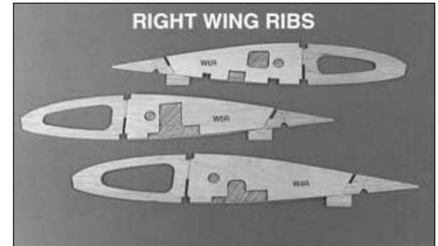
**R2.** Prepare a set of **right** wing ribs by using 30-minute epoxy to glue the die-cut 1/16" [1.6mm] plywood **retract landing gear rib doublers W4R, W5R and W6R** to the die-cut 3/32" [2.4mm] balsa **ribs W4, W5 and W6 exactly** as shown in the photo. Make sure the doublers are on the side of the ribs as shown in the photo and on the right wing plan.
