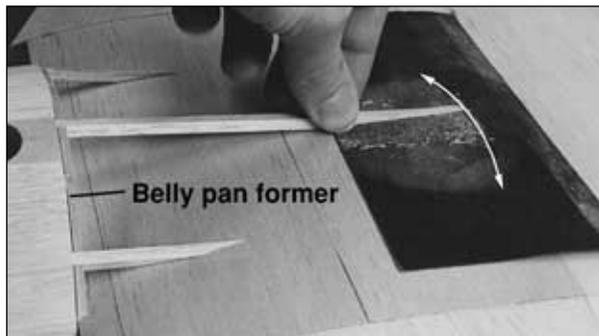
❑ 2. From a 3/16" x 3/16" x 30" [4.8 x 4.8 x 762mm] balsa stick, cut one 6-1/2" [165.1mm] piece, two 4-3/4" [120.7mm] pieces and two 2-1/4" [57.2mm] pieces to make the **belly pan stringers**. Sand one end of the stringers so they conform to the shape of the bottom of the wing. Glue them in position.
