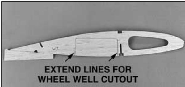
**R6.** Use a ballpoint pen to *extend* the die-cut *wheel well cutout* in both W3 ribs. Cut partway through the rib along the line so the cutout will be easier to remove later.
