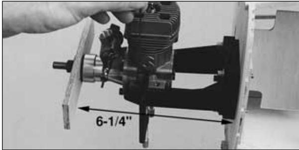
❑ 11. Mark the engine mounting bolt holes on the mount. **Hint:** Mark the holes with a wire rod sharpened at one end. Heat the tip of the rod with a torch to dimple the engine mount in the **center** of the holes. The Great Planes Dead Center Tool (GPMR8130) also works well.
