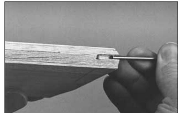
□ 50. Drill a 9/64" [3.6mm] hole 1-1/4" deep and cut a groove in the center of both LE's for the joiner. Test fit the elevator joiner in the elevators.
