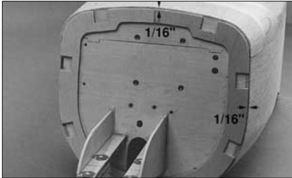
❑ 4. Test fit the die-cut 1/8" [3.2mm] plywood **cowl rings** on the firewall. If necessary, sand the edges of the cowl rings so they are inset from the edges of the balsa fuselage sides approximately 1/16" [1.6mm]. Glue the cowl rings to the firewall.
