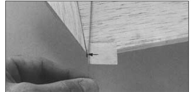
❑ 3. Tie a loop on one end of a 54" [1372mm] piece of string and connect it to the T-pin in the top of the firewall. Put a piece of masking tape with an arrow on it near the other end of the string. Slide the tape along the string and align the arrow with the corner of one of the stab halves. Swing the tape over to the other corner on the other side of the stab. Shift the stab and slide the tape along the string until the arrow aligns with both corners of the stab.
