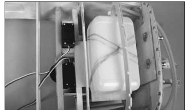
❑ 1. Assemble your fuel tank. Position the tank floor and the tank in the fuselage and determine where to
