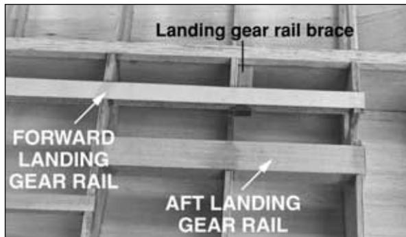
❑ ❑ R7. Cut the 1/2" x 3/4" x 6-3/4" [12.7 x 19 x 172mm] grooved basswood **aft landing gear rail** to a length of 6-1/8" [155.6mm]. Test fit, then glue the rail in position with 30-minute epoxy (**with the groove facing the top sheeting**). Test fit, then glue the 1/4" x 1/2" x 9" [6.4 x 12.7 x 229mm] plywood **forward landing gear rail** in position with 30-minute epoxy. Immediately proceed to the next step before the epoxy cures.
