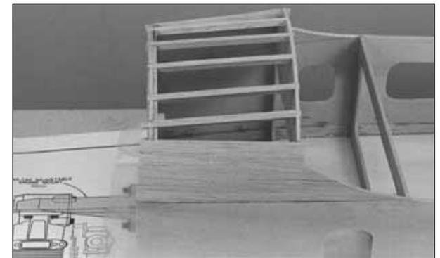
❑ 1. Refer to the photo in the following step and test fit a die-cut 1/8" [3.2mm] balsa **forward fuse doubler** on the right side of the fuse. The front edge of the forward fuse doubler should align with the front edge of the fuse side doubler. Wet the outer surface of the doubler and glue it in place. Be sure that former F2 remains square and flat.
