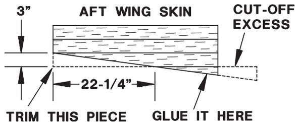
❑ 1. Glue **three** 3/32" x 3" x 36" [2.4 x 76 x 914mm] balsa sheets together to make an **aft wing skin**. Trim a *wedge* from the aft wing skin. Glue it back onto the skin as shown in the sketch.
