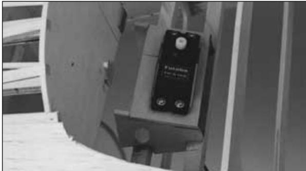
❑ R9. Cut 3/16" [4.8mm] off the aft edge of the die-cut 1/8" [3.2mm] plywood **nose steering servo tray**. Mount your nose steering servo to the servo tray, using the hardware that came with the servo, so the output shaft is on the **left** side of the servo tray as shown in the photo. Note that the servo is offset toward the aft edge of the servo tray (the side you cut off).
