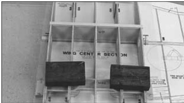
❑ 12. Pin small blocks of leftover balsa to the plan next to the W1 ribs, aligning them over the plan, and place weights on top of the ribs and spars to hold the jig tabs to the building board. Use a small square to make sure the W1 ribs are vertical.
