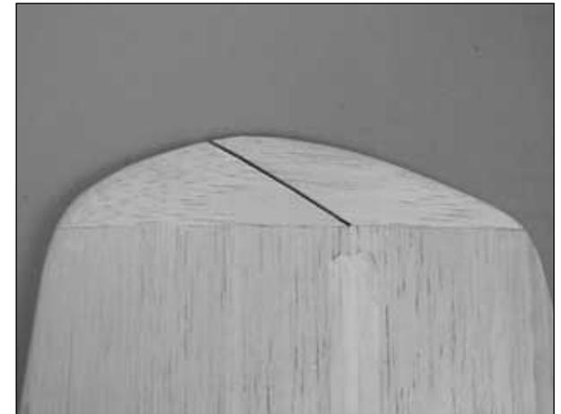
❑ 29. Use thick or medium CA to glue the rudder and fin tip blocks to the rudder and fin in the same manner that you glued the tip blocks to the elevator and stab. Use the centerline on the tip blocks as a guide to make sure it is centered on the rudder and fin.
