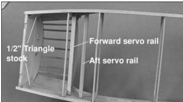
❑ 3. Cut a 8-3/4" [222.3mm] **aft servo rail** to fit between the fuselage side doublers 7/8" [22.3mm] aft of the forward servo rail. Place the throttle and nose wheel steering servos and trays between the rails. Adjust the position of the aft rail to fit your servos. Glue the aft servo rail in place. **Do not** glue the servo trays in place until instructed to do so.
