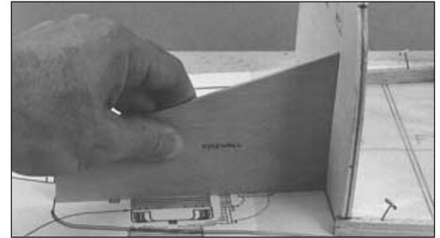
❑ 6. Glue the firewall to the side stringers using the die-cut 1/8" [3.2mm] plywood **firewall angle gauge** to hold the firewall at the correct angle. This will establish the correct down thrust for the engine.
