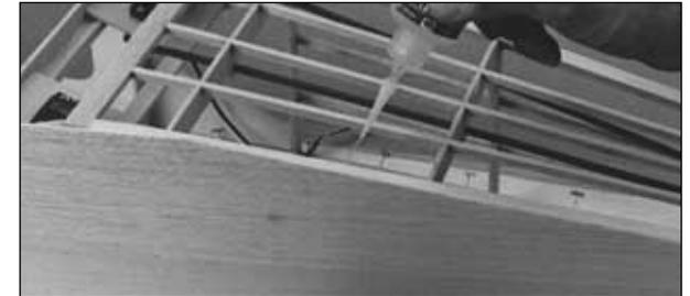
❑ ❺ 5. Apply a bead of medium CA to the *step* portion of the stepped balsa side stringer from the firewall to former F6. Working quickly, position the side sheet on the ledge of the side stringer and press it into position where you have applied the glue. After the CA dries apply thin CA to the side stringer and side sheet aft of former F6 from inside the fuse. A long CA applicator tip, such as the Hobbico applicator tip (HCAR3780), helps you apply the CA just where you need it.
