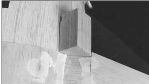
❑ 4. With the wing off the fuse, sand one of the 1-3/8" x 1-3/8" x 1-1/2" [35 x 35 x 38.1mm] **wing fairing blocks** to match the curvature of the right side of the fuse at the leading edge of the wing. Bolt the wing to the fuse. Sand the side and rear of the wing fairing block so it fits between the wing and the fuse as shown in the photo. Glue the wing fairing block **to the wing only**.
