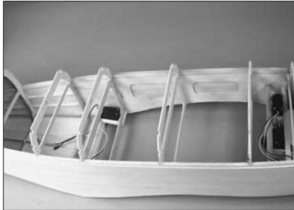
❑ 5. Glue the die-cut 1/8" [3.2mm] plywood formers **F3A** through **F6A** in place as shown on the plan. The formers are glued to the front of its corresponding former. If you previously cut slots for the servo wires in F3, F4 and F5, then cut the needed slots in F3A, F4A and F5A.
