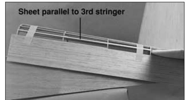
❑ 5. Cut one of the bottom turtle deck sheets to a length of 21-1/2” [546mm]. Position the sheet on the left side of the turtle deck so the top edge contacts the bottom of the stab and is parallel to the third stringer from the bottom as shown in the photo.
