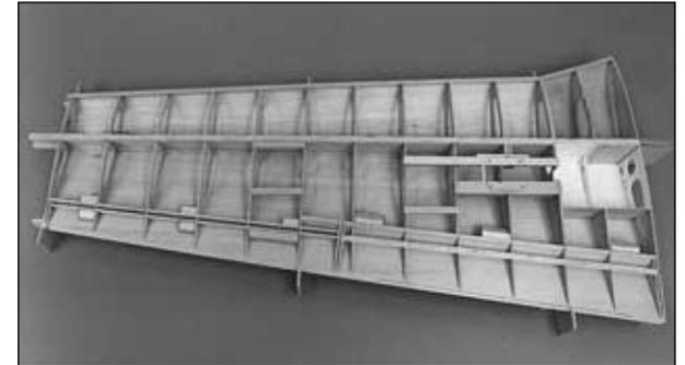
❑ 5. Place the wing on your workbench so it is resting on the cradles. Fit the bottom sheeting to the wing. Trim the *stoppers* on the cradles so the trailing edge of the bottom sheeting aligns with the trailing edge of the top sheeting. Trim the front edge of the sheeting so it *ends* at the center of the spar (the same way as the top sheeting).
