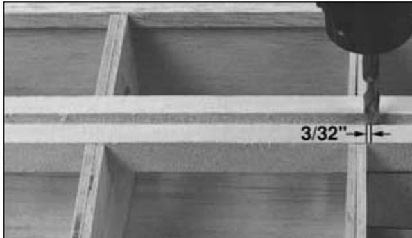
□ □ F16. After the epoxy on the landing gear rail has fully cured, drill a 3/16" [4.8mm] hole through the landing gear rail and the torque block. The center of the hole should be 3/32" [2.4mm] from the plywood rib doubler W4G. Make sure you hold the drill perpendicular to the bottom of the landing gear rail.
