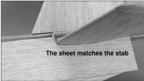
□ □ 7. Reposition the sheet so that it rests against the bottom of the stab. Mark and cut it along the line. Do this until the sheet accurately matches the bottom of the stab.
