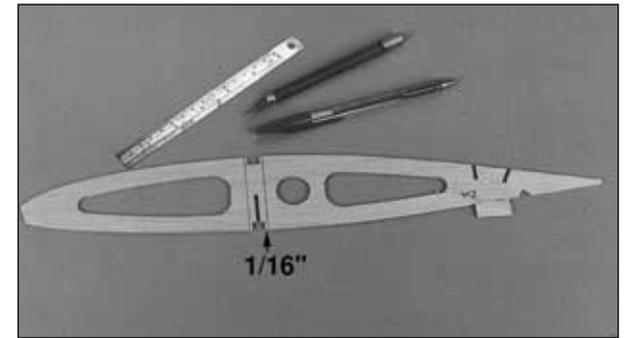
□ 11. Use a straightedge and a ballpoint pen to mark a vertical line 1/16" [1.6mm] from the front and back of the spar notches in both **W2 ribs**. Use a sharp hobby knife to **lightly** cut halfway through the balsa along the lines. You will remove this section of balsa to accommodate the spar joiners when it is time to join the wing.
