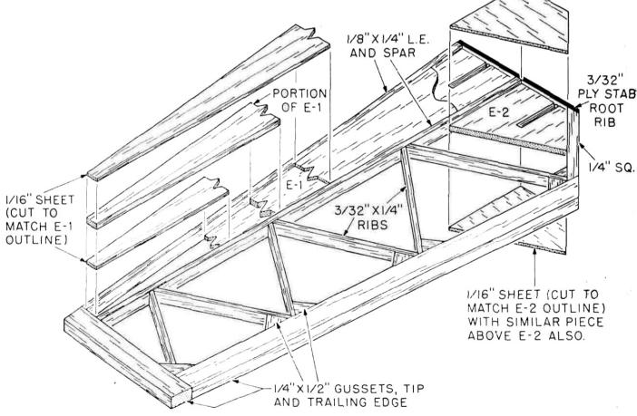
note that the "entry" or leading edges are not particularly sharp, but not just "rounded" either. Approach thistaskwith care tocreate the intended shapes. Final sand with light paper and set aside for covering.
