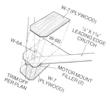
4. Remove the leading edge crutch from the plans, turn it over and use your sanding block to smooth out any glue joints. Glue the remaining W-7 part in place to the bottom surface of the crutch assembly, exactly aligned with the W-7 previously glued to the top surface. Again, use weights to hold this part in place and allow it to dry.
