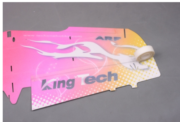
2. Use 3M magic tape to splice the two ailerons and the wing.
