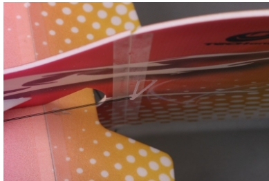
39. Link the servos and elevator control horns with threads. Make sure the threads are taut and the two ends of the servo arms are tied with threads.
