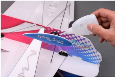
29. Fix the wheel covers to the wheels with some C/A.
