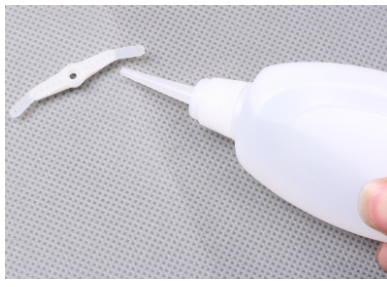
33. Glue 1pc bended fiber glass and 1pc original servo arms together. (for aileron)
