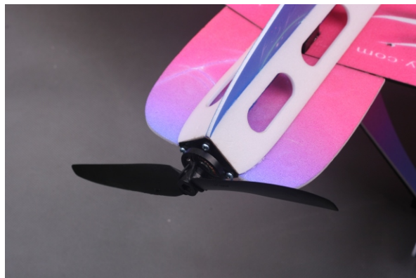
48. Install the propeller.
