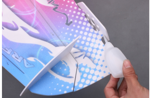
43. Insert the aileron damping board into pre-reserved place, then apply some foam friendly C/A to fix it.
