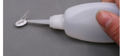
34. Glue together the control horns and their backplates. (for aileron)
