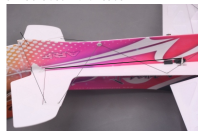
39. Link the servos and elevator control horns with threads. Make sure the threads are taut and the two ends of the servo arms are tied with threads.
