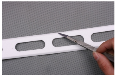
27. Bevel 45 degree the fuselage stringers.
