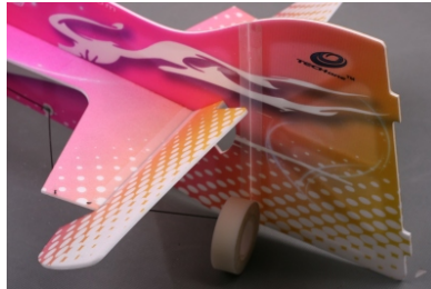
23. Fix the rudder to the fuselage with 3M magic tape.
