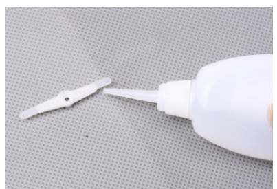
32. Glue 1pc straight fiber glass and 1pc original servo arms together. 2 kinds of fiber glass servo arms, straight servo arm (2pcs) and bended servo arm (1pc).
