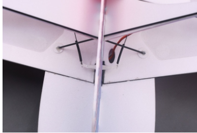
37. Install aileron carbon fiber rods.
