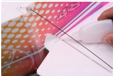
26. Install the elevator and rudder control horns.
