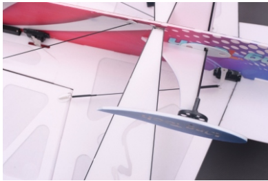
37. Install aileron carbon fiber rods.
