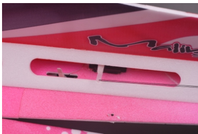
39. Link the servos and elevator control horns with threads. Make sure the threads are taut and the two ends of the servo arms are tied with threads.
