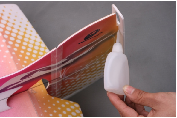
44. Install the rudder damping board. Same assembly as the aileron damping board.
