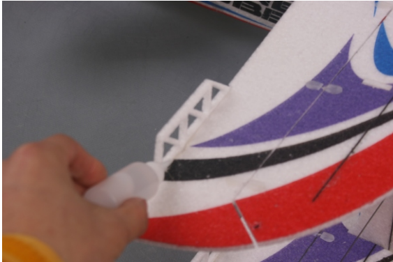
Glue the spoiling flap to the wing.
