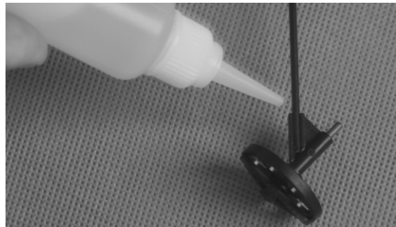
Install the two wheels and wheel chocks. Keep 1mm distance between wheel and its chock. Apply some foam-friendly thick C/A to glue the chocks.
