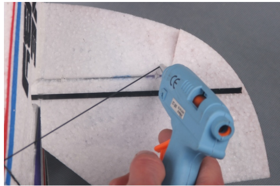
Glue the two carbon fiber rods to the stabilizer.
