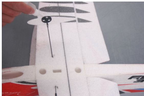
Slide one wheel cover onto each axle and up against the wheels. Align the wheel covers, then glue them securely to the axles.
