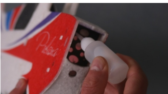
Apply some foam-friendly C/A into the four motor mount screw holes in the firewall.
