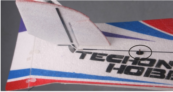
Install the elevator control linkage(380mm).
