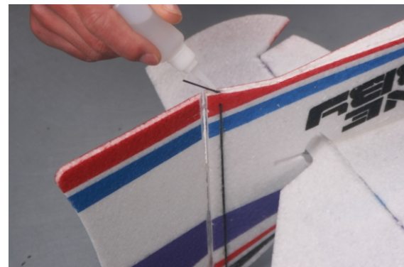
Cut one piece of carbon fiber rod of 50mm, then insert it to the fuselage and glue it.
