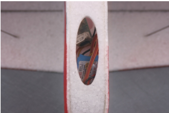
Mount your ESC and receiver, using a piece of hook and loop material.
