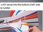
Cut the two carbon rods. One end of the carbon rod is fixed into the hole of the fin with some glue and the other end is fixed into the hole of the fuselage. Make sure they are vertical.
