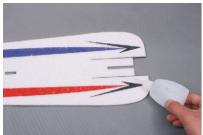
insert two 100mm long carbon strip into the precutting slots of the horizontal fuselage head, fixed with some glue.
