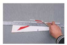
Cut a 45 bevel into the bottom leading edge of the ailerons.
