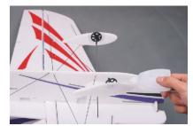
Slide one wheel pant onto each axle and up against the wheels, Align the wheel pants. Then glue them securely to the axles.
