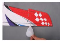
Cut a piece of carbon fiber strip to a length of 762mm, insert it into the precutting slot of the wing and fix it with glue
