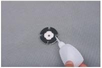
Glue the firwall to the EPP motor doubler with C/A glue.
