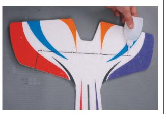
Insert the hinges into the precutting slot of the stabilizer and fix them with glue. Then hinge the elevator to the stabilizer with some glue.
