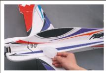
Key the top vertical fuselage to the horizontal fuselage, using some glue. Before glue the joints, please make sure the vertical fuselage is perpendicular to the horizontal fuselage.
