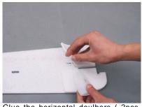
Glue the horizontal doulbers (2pcs EPP strengthen plates) to the underside of the horizontal fuselage as shown
