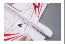
Install and Locate the Landing gear. thread the Landing gear through the vertical fuselage and into the horizontal fuselage. Be careful, Do Not press the landing gear all the way through the horizontal fuselage. Glue the landing gear in place using some glue.
