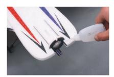
put the motor mount onto the firewall and drill the screw holes. sticking the drilled hole firewall with the head of plane
