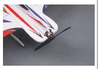
Assemble the motor onto the firewall, using the four wood screws provided. PRO TIPAfter flying the airplane, you may want to add right and/or down thrust to the motor. You can do this by adding thin washers between the motor mount and the firewall.
