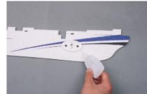
Locate the two Epp landing gear mounting plates . Glue a landing gear plate to each side of the fuselage in the location shown.
