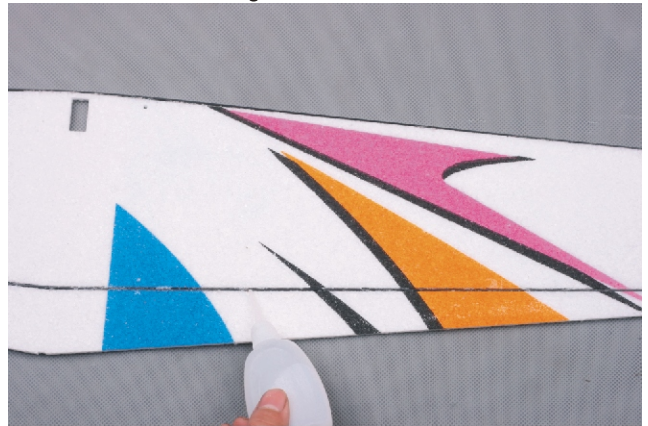
Put the carbon slice into wing, use some glue to stick.
