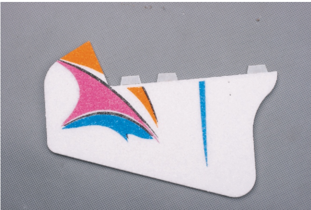
Apply a thin layer of glue to each hinge, then insert them into the slots.
