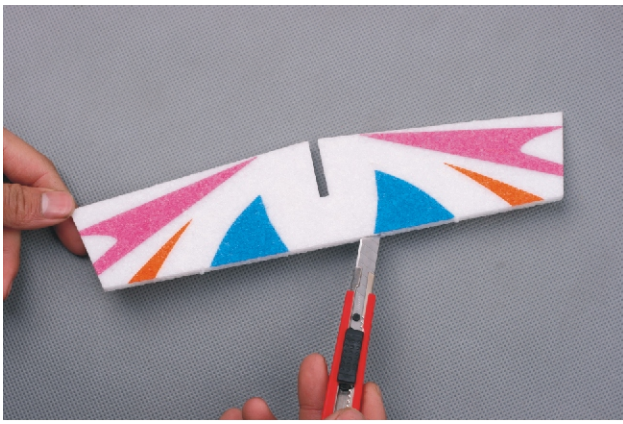
Cut 4 hinge slots in corresponding locations of the horizontal stabilizer.
