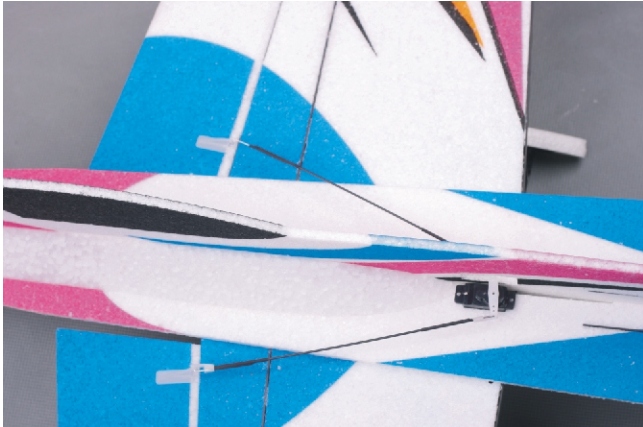
Center the aileron servo, then attach the servo arm onto the servo, making sure that it is centered. Check that servo arm is still centered, then center both ailerons. Cut the pushrod wires to length, snap the clevises into the outermost holes in the control horns, then glue the clevises to the pushrod wires.
