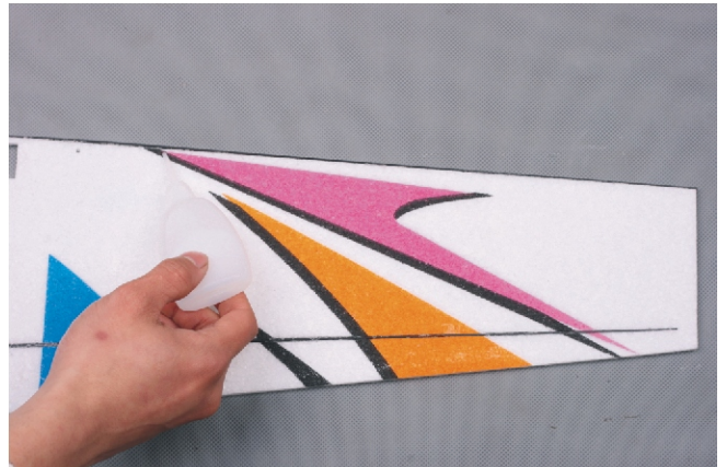
Put the carbon slice into leading edge of wing and stick with some glue.
