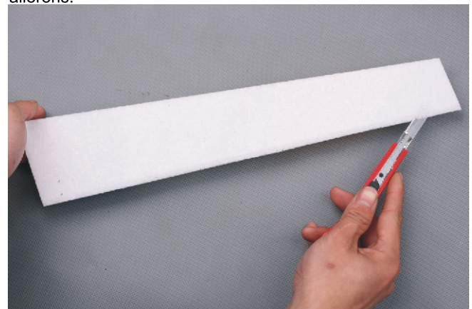
Cut 4 hinge slots in the leading edge of the ailerons.
