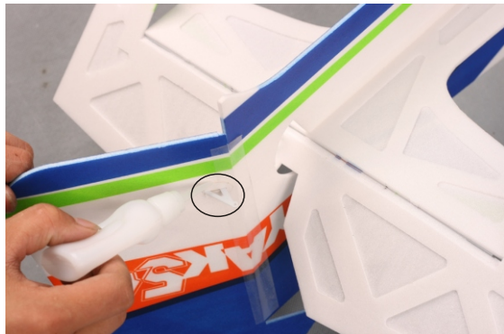
Fix the rudder control horns with some C/A.
