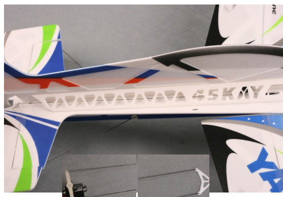
Link the servos and control horns with threads, make sure the threads are taut and the two ends of the servo arms are tied with threads.
