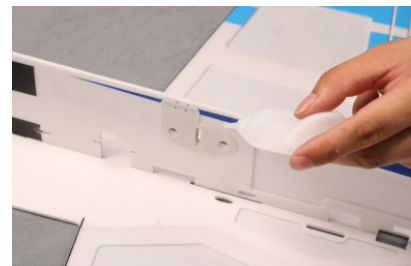
Install the doubler for the landing gear.
