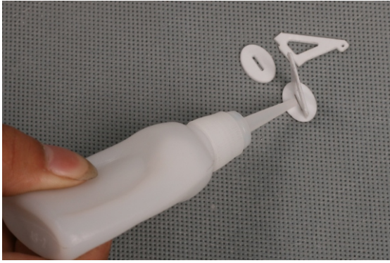
Glue together the control horns and their backplates.
