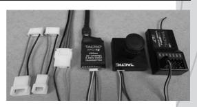
information. To power the camera, plug the connector into the receiver or another 4.8~5V source. Do not exceed 5V or you risk damage to the camera. Check the specs of your ESC to confirm the voltage.
