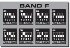
BAND SELECTION: Switches 4 and 5 are used to set either band A, B, or F. Place both switches UP for band A, switch 4 down and switch 5 up for band B, and both switches DOWN for band F.
