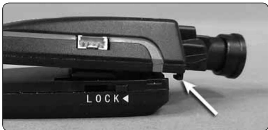
Push the camera forward and up from the module to release the front catches.
