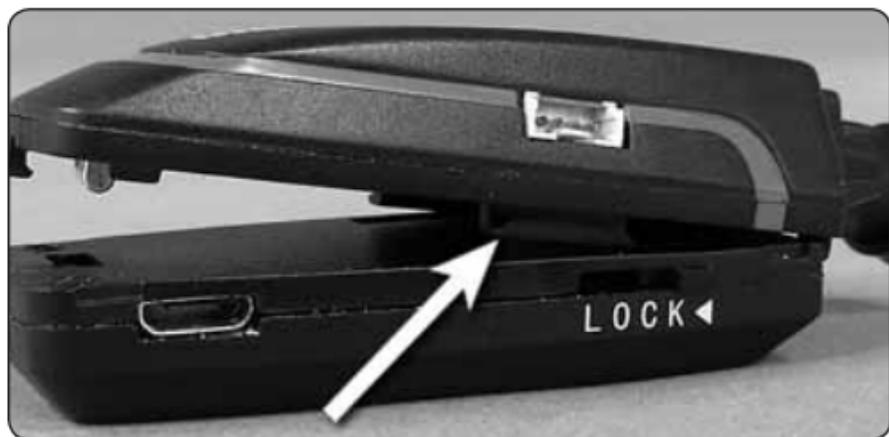
Slowly raise the back of the camera until the tabs are clear of the battery module.
