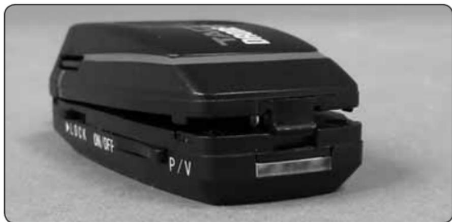
Carefully pull up on the tab at the back of the camera.
