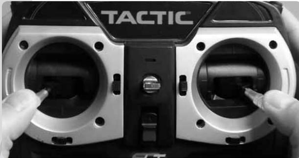
1. With the Tx power switch off, move the right stick to the bottom-right corner, the left stick to the bottom-left corner, and hold in these positions.
