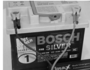
Using terminal clip attaching to car battery
