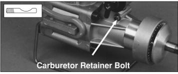
Insert the carburetor retaining bolt (the bolt has a curved area removed from its center) into the hole in front of the carburetor opening. Rotate the retaining bolt so that the removed area in the bolt matches the curve of the carburetor opening. Install the split washer and the brass nut on the threaded end of the bolt. Insert the carburetor in the carburetor opening and press down on the carburetor while tightening the nut.
