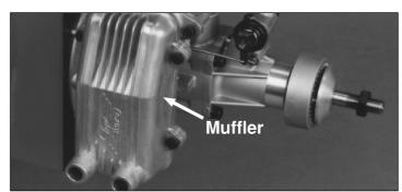
Install the 5mm-.8 screw, split washer and 5mm nut in the muffler, but do not tighten. Slide the muffler over the exhaust manifold and position it so that it does not touch the fuselage. Also, to reduce drag it is best to position the muffler parallel to the fuselage. When the muffler is positioned correctly, tighten the 5mm-.8 screw to clamp the muffler over the exhaust manifold.
