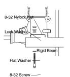
Set the engine on the beams at the correct angle to the centerline of the fuselage, according to the instructions provided by the airplane manufacturer. When the engine is mounted in the upright position, the centerline of the fuel tank should be at the same level as the high speed needle, or no more than 3/8" lower, to
