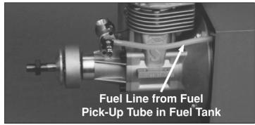
Connect a medium or large size silicone fuel line from the fuel inlet on the carburetor to the fuel pick-up tube that is connected to the clunk in the fuel tank. We suggest that a fuel filter be installed in the fuel line between the carburetor and the fuel tank. The filter will prevent any contaminants in the fuel from clogging the carburetor and doing damage to the internal parts of the engine.
