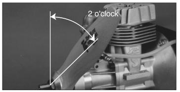
Continue rotating the propeller until it's at the 2 o'clock position, then tighten the propeller nut **securely** against the propeller washer. Some people use a 4-way wrench for this purpose, but it is difficult to get the nut tight enough with that type of wrench. Many modelers use (and we recommend) a 6-inch adjustable wrench for tightening prop nuts.
