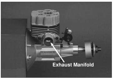
Use two 4mm-.7 size screws and split washers to attach the exhaust manifold to the engine. Make sure to install the gasket between the manifold and the engine and tighten the screws securely.
