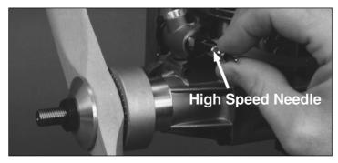
4. Gently turn the high-speed needle valve clockwise until it stops. Do not tighten it. Then open it 4 turns. Turning the high speed needle in a clockwise direction is called "leaning" the mixture, and turning it counterclockwise is called "richening" the mixture.
