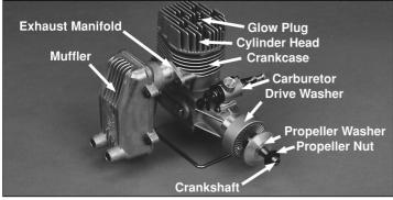
**Crankshaft:** The crankshaft transforms the reciprocating motion of the piston into rotational motion. The propeller is mounted on the portion of the crankshaft protruding from the crankcase. The portion of the crankshaft protruding past the drive washer is known as the "prop shaft."
