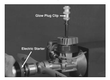
**Securely** attach the glow plug clip to the glow plug. If using a glow plug clip connected to the power panel of a field box, make sure the wire cannot become entangled in the propeller.
