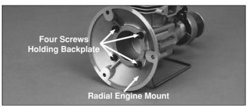
If the engine is to be mounted on the radial mount provided with the engine, remove the four screws holding the backplate. Remove the rubber O-ring on the backplate and install it on the radial mount. Attach the radial mount to the engine using the four longer screws
