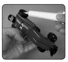
**4.** Apply graphite powder<sup>3</sup> between the inside of the axle head and outside of the wheel. Slowly turn the wheel and shake the car to work the powder into the wheel.
