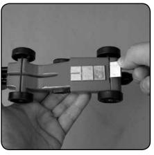
**2.** Attach the weight to the bottom of the car with double sided foam tape.
