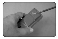
1. Clean all dust from the body. Apply a thin coat of paint as evenly as possible. When dry, use fine sandpaper to lightly scuff the paint. Apply additional coats
