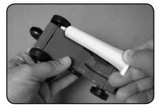
**5.** Apply graphite powder<sup>3</sup> to the inside of the wheel where it makes contact with the body.
