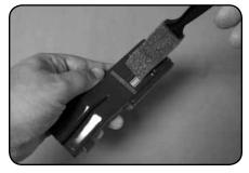
**3.** Use a foam brush to apply an even layer of clear coat. Extra layers can be applied if needed.
