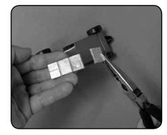
1. Weigh the car with all the parts installed. Use a pair of pliers to break off as many sections of weight as needed to meet the 5 oz (141 gram) limit.
