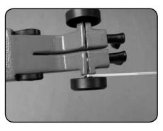
2. Space each wheel to have a small gap. Place the wheel adjustment tool<sup>2</sup> between the body and the wheel. Move the axle and wheel until the tool fits snugly between the
