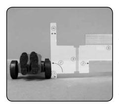
**3.** Place the car on a smooth, flat surface. Place a wheel adjustment tool<sup>2</sup> with the camber check section against the face of the wheel. Adjust each axle to make the wheels parallel to the edge of the adjustment tool.
