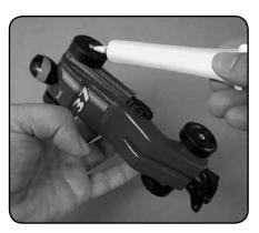
**4.** Apply graphite powder<sup>4</sup> between the inside of the axle head and outside of the wheel. Slowly turn the wheel and shake the car to work the powder into the wheel.
