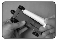
**5.** Apply graphite powder<sup>4</sup> to the inside of the wheel where it makes contact with the body.
