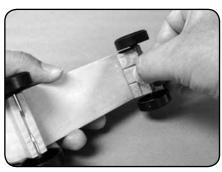
**2.** Attach the weight to the bottom of the kit using the double sided foam tape.
