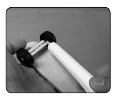
**5.** Apply graphite powder<sup>3</sup> to the inside of the wheel where it makes contact with the body.
