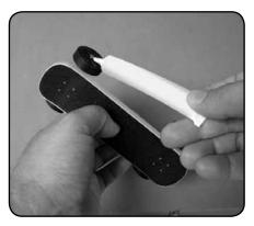
**4.** Apply graphite powder<sup>3</sup> between the inside of the axle head and outside of the wheel. Slowly turn the wheel and shake the kit to work the powder into the wheel.
