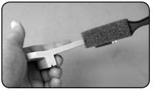
**3.** Use a foam brush¹ to apply an even layer of clear coat.¹ Extra layers can be applied if needed.
