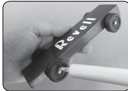
**4.** Apply graphite powder between the axle head and wheel. "Work in" the powder by shaking the car and slowly turning the wheel.
