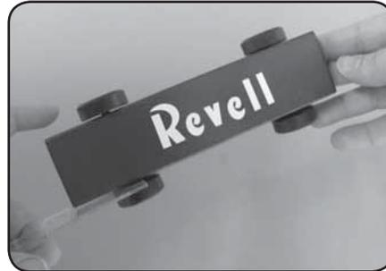
**2.** Slide a wheel adjustment tool between the wheel and body. Move the wheel until the tool fits snugly.
