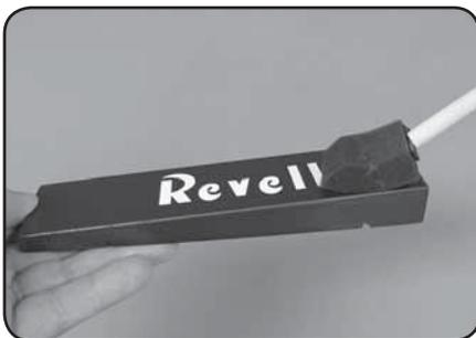
**4.** Apply an even layer of clear coat with a foam brush. Apply more layers as needed.
