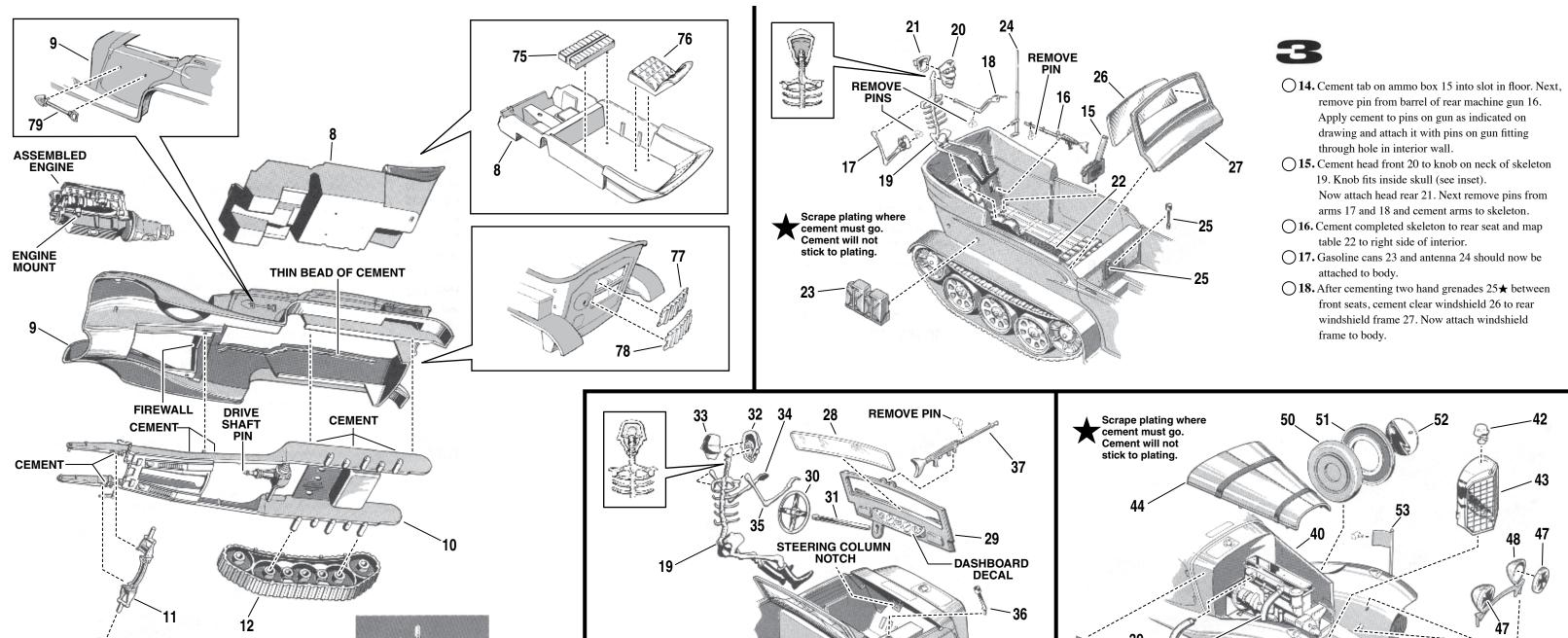
**6.** Apply cement to two pins on shovel 79 and insert into holes on body 9. Next, apply cement to pins on ammo box 75 and seat 76 then insert into holes in interior 8.
