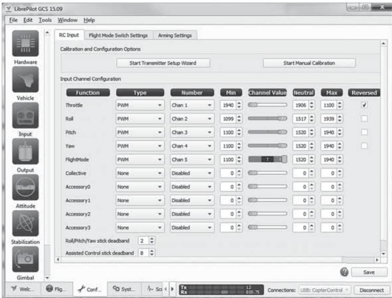
At the end of the wizard is the screen to set the motor arming procedure. The recommended setting is Yaw Right which requires the yaw control to be held to the right while the throttle is at 0 for 3 seconds. Holding the Yaw control to the left will disarm the motors. There are several other options available for arming/stopping the motors including using a switch assigned to Channel 6.
