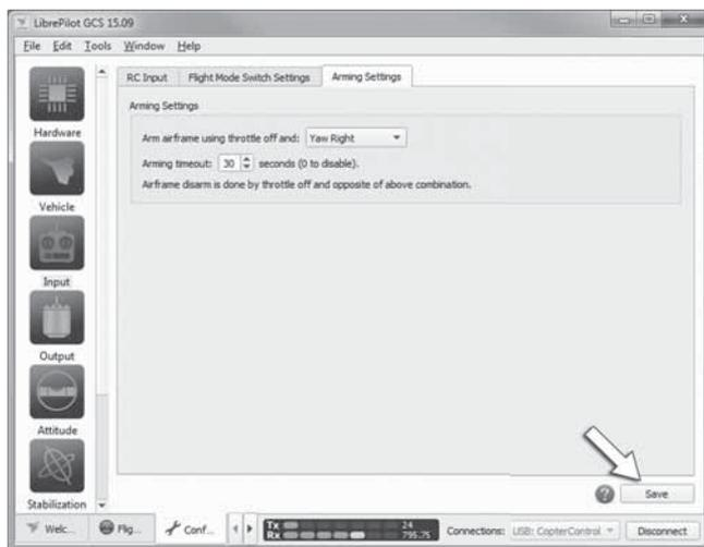
After the Arming Setting is selected, the settings need to be saved to the flight controller
