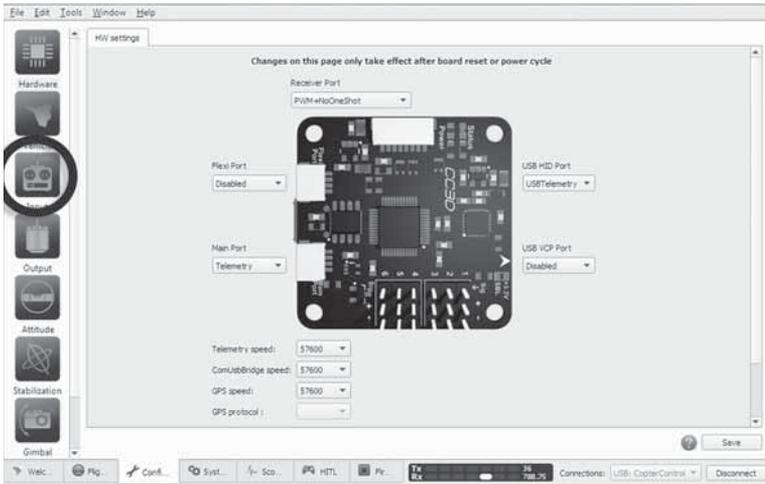
If your transmitter and receiver have already been setup with the flight controller, this page can be used to test the transmitter controls and switches. The flight battery will have to be connected to power the receiver. Warning: Remove the props before connecting the flight battery to the quadcopter.
