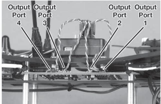
The 5V power cable should be plugged into Output port 5 or 6 with the brown wire in the “-” column.
