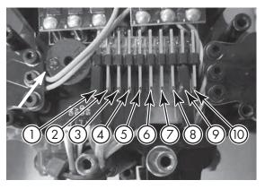
If an S.Bus receiver is being installed, the cable from the receiver should be plugged into the adapter's Channel 9 port. The PPM cable goes to Channel 10.
