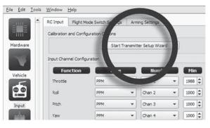
At the end of the wizard is the screen to be used to set the motor arming procedure. The recommended setting is Yaw Right which requires the yaw control to be held to the right while the throttle is at 0 for 3 seconds to arm the motors. Holding the
