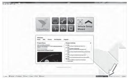
Open the GCS app and connect the RXD250 with your mini-USB cable. When the communication window shows that the flight controller is connected to the GCS app, click on the configuration button.
