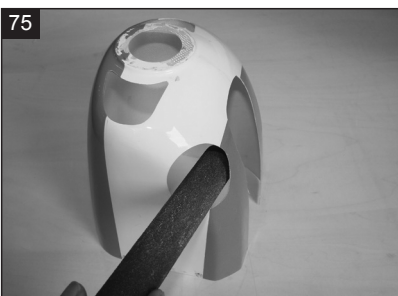
75 Make the hole for the engine, the muffler.
