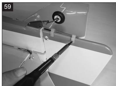
59 Secure the nylon keeper.
