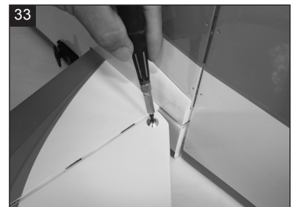
33 Install the control horn.
