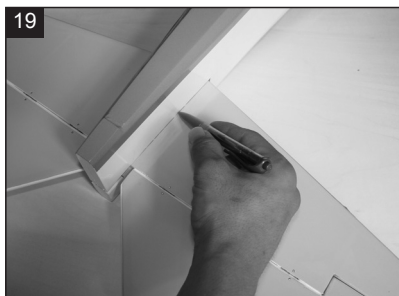
20 And mark the shape of the fuselage onto the bottom of the horizontal.
