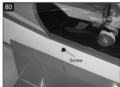
80 Secure the canopy to the fuselage.
