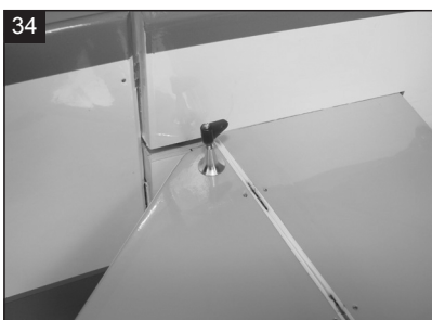
34 Install the nylon horn.
