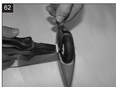
62 Install the wheel pant.
