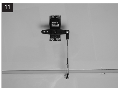
Attach the metal clevis to the nylon control horn.
