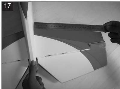
17 Insert the horizontal into the fuselage.
