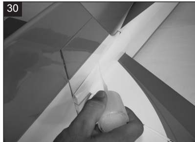
30 Glue the vertical using the epoxy glue.
