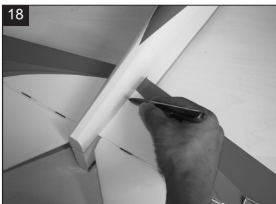
19 Mark the shape of the fuselage onto the top of the horizontal.
