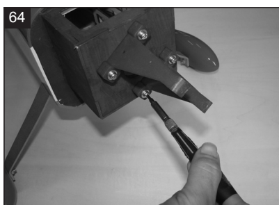
64 Install the engine mount to the fuselage.
