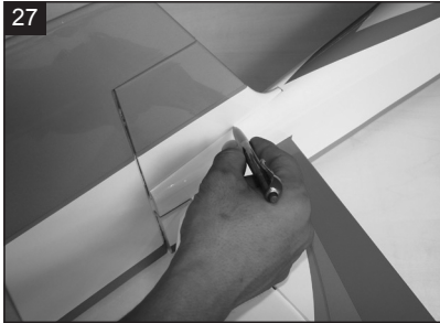
27 Mark the shape of the fuselage onto the vertical.
