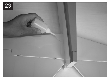
24 Glue the horizontal to the fuselage using the epoxy glue.
