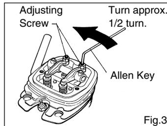
3. Insert 0.04mm feeler gauge between valve stem and rocker-arm and gently turn adjusting screw clockwise until it stops.(Fig.4.)
