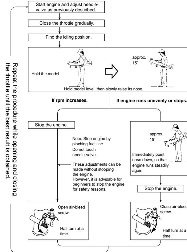
**Attention: Do not leave the glowplug connected to the battery while adjusting the carburetor throttle.**
