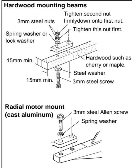
Make sure that these mounting beams are accurately aligned and firmly integrated with the airframe, reinforcing the adjacent structure to absorb vibration. Use 3mm or larger steel screws, preferably Allen type hexagon socket head cap screws, with washers and locknuts, for bolting the engine to the bearers.
