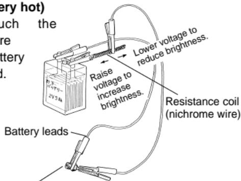
Adjust applied voltage by changing the position of clip on resistance coil until glowplug element is glowing bright red.
