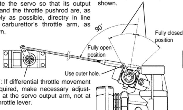
**Note** : If differential throttle movement is required, make necessary adjustment at the servo output arm, not at the throttle lever.
