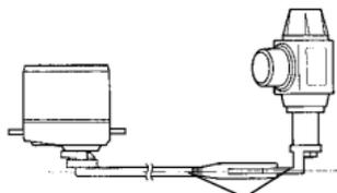
Locate the servo so that its output arm and the throttle pushrod are, as closely as possible, directly in line with carburetor's throttle arm, as shown.
