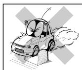
"no load" conditions (i.e. with the driving wheels not in contact with the ground) it will rapidly over-heat and may be seriously damaged.
