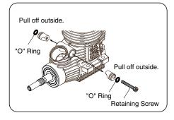
Make sure that the vehicle's engine mounting surfaces are level and in the same plane. Poor installation may cause distortion of the crankcase, bearings, etc., resulting in erratic running and loss of performance.
