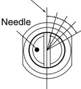
Close the needle-valve approx. 15° after running the vehicle for 1 to 2 full tanks of fuel. Repeat this procedure until approx. 2 liters of fuel have been consumed.
