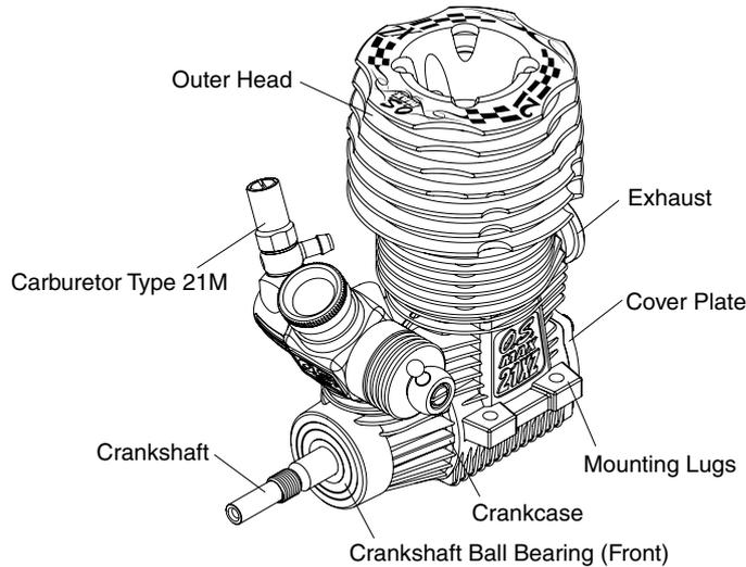
Installing the glow plug. Insert RP7 plug supplied into heat-sinkhead carefully, making sure that it is not cross-threaded before tightening firmly. (All the O.S. T-Type plugs including the RP7 are not supplied with a washer.)
