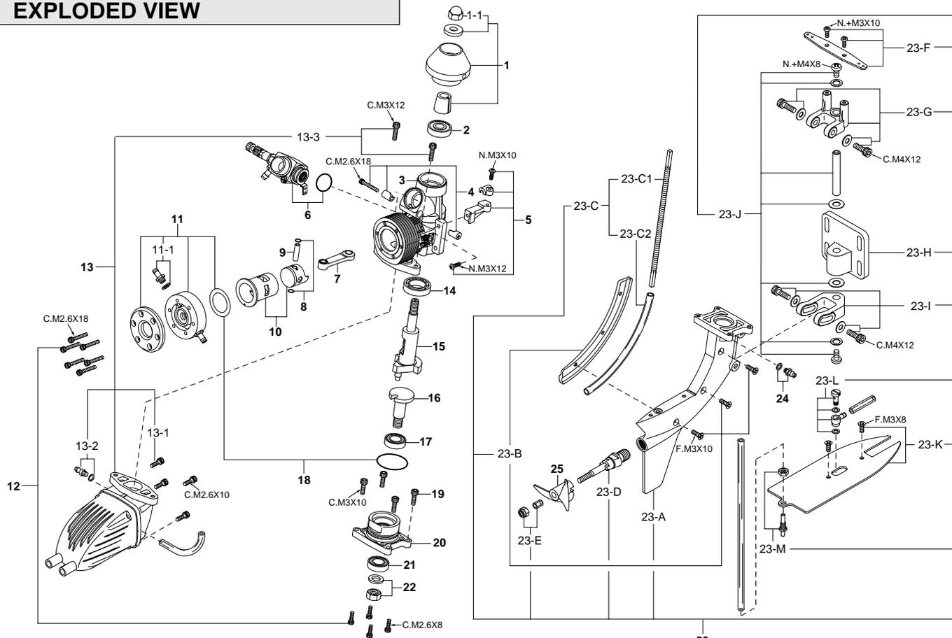
\* Type of screw C···Cap Screw M···Oval Fillister-head Screw F···Flat Head Screw N···Round Head Screw S···Set Screw
