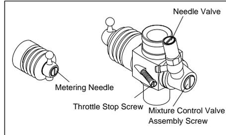
**NOTE: Readjustment may be necessary, occasionally to allow for changes in fuel formula gear ratio or clutch engagement point.**
