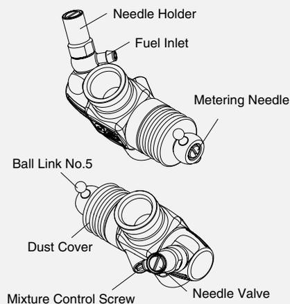
Three adjustable controls are provided on this carburetor.
