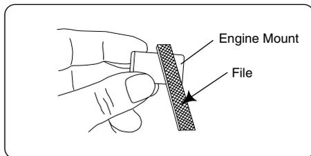
Make sure that the vehicle's engine mounting surfaces are level and in the same plane. Poor installation may cause distortion of the crankcase, bearings, etc., resulting in erratic running and loss of performance.
