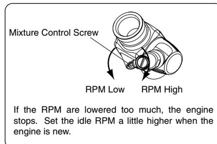
If the RPM are lowered too much, the engine stops. Set the idle RPM a little higher when the engine is new.
