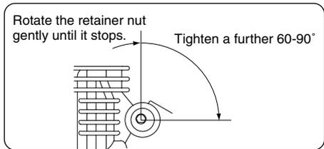
2. Rotate the retainer screw gently until it stops, then tighten a further 60-90°. Do not overtighten the screw as this will damage the carburetor body.
