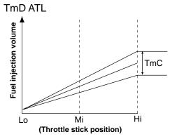
This adjustment mechanism allows adjustment of a single trim point using the slow position as the origin. Adjustment uses the injection trim adjustment dial (spare channel dial) on the transmitter. There is no change at Lo (slow position) while the trim volume reaches a maximum at Hi.
