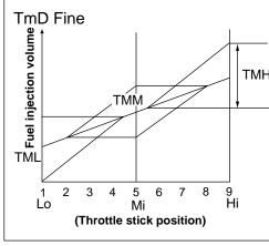
Injection trim can be adjusted independently for three points (TmL, TmM and TmH) as shown in the graph. Mi (intermediate slow TmM) and Hi (full high TmH) are adjusted with the injection trim adjustment dial (spare channel dial) on the transmitter. Lo (full slow TmL) is adjusted on the TRL menu displayed following the function menu.
