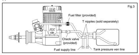
Connect all lines securely as shown in the figure above. Since high pressure is applied to the fuel tank from the engine crankcase, make connections using a commercially available, thick-walled silicon tube. In addition, make sure to securely seal the area around the cap. If the outlet of the T nipples is left accessible from outside the airplane, it will make venting tank pressure and refueling easier. Always make sure to use the check valve and fuel filter provided.
