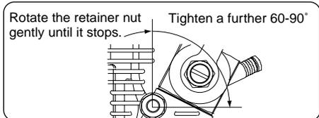
2. Rotate the retainer screw gently until it stops, then tighten a further 60-90°. Do not overtighten the screw as this will damage the carburetor body.
