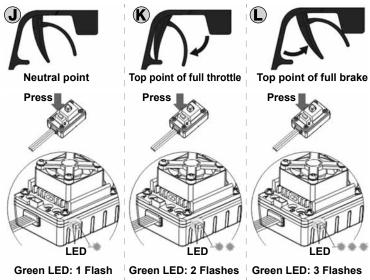
J. With the Tx trigger at the neutral point, press the SET button. The green LED will flash once to indicate the setting point has been accepted.
