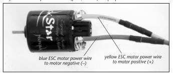
4. CHECK FOR PROPER GEARING DURING INITIAL RUNS The brushless motor & ESC should NOT get hotter than 160°F--Crawler motors/ESCs generally DO NOT get very hot. Reduce pinion size and check the drive train for binding if you experience high operating temperatures.
